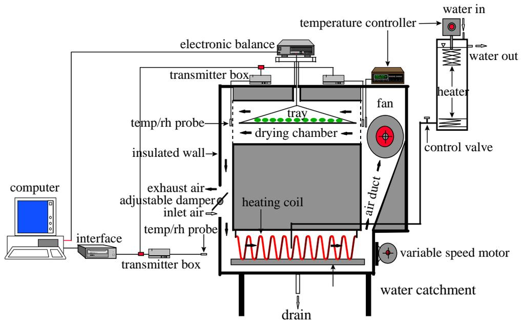
Figure 1: Schematic diagram of the dehydration system
