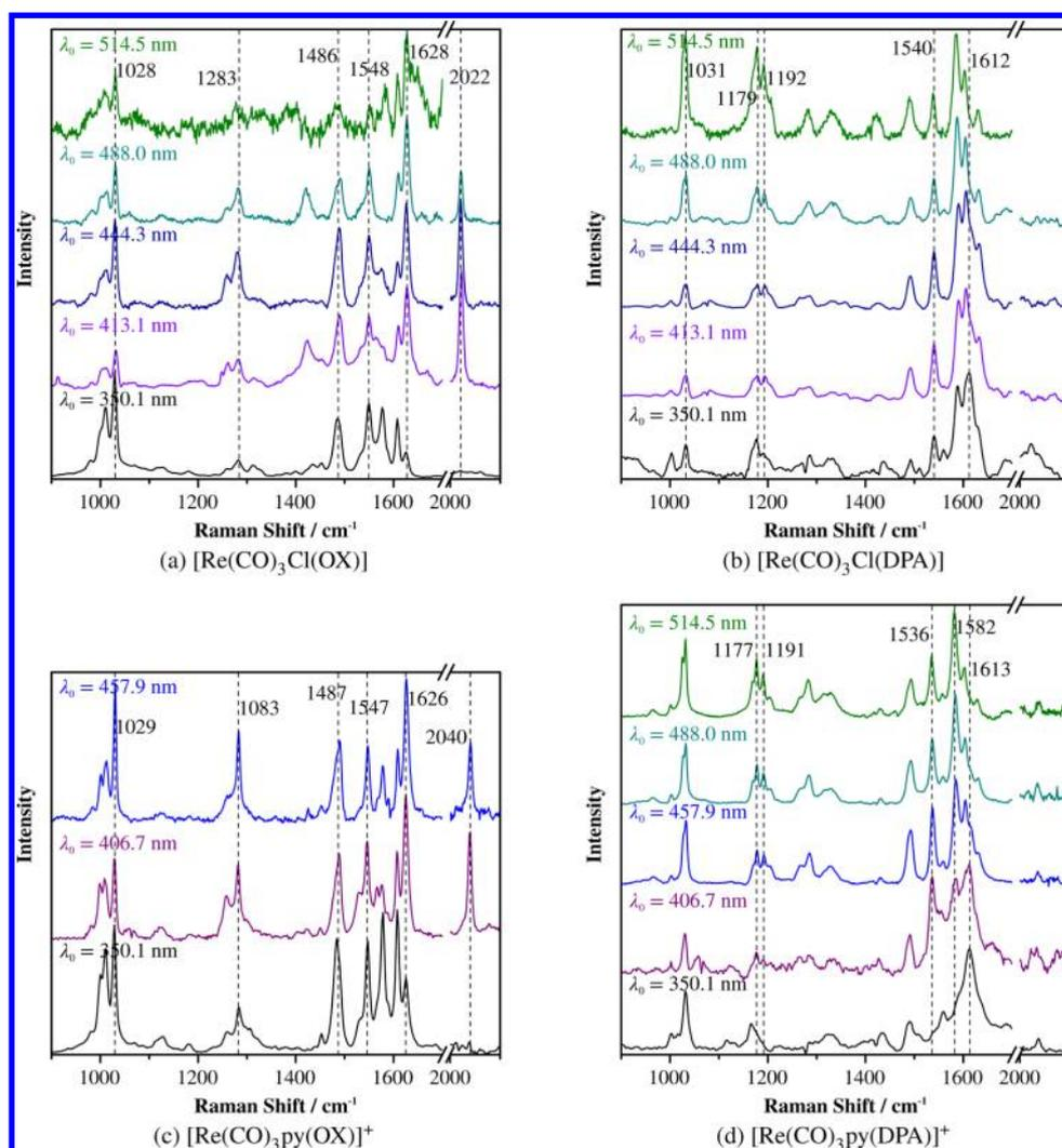
**Figure 8.** Resonance Raman spectra at a number of excitation wavelengths: (a)  $[\text{Re}(\text{CO})_3\text{Cl}(\text{OX})]$  acquired in DMSO, (b)  $[\text{Re}(\text{CO})_3\text{Cl}(\text{DPA})]$  acquired in DMSO, (c)  $[\text{Re}(\text{CO})_3\text{py}(\text{OX})]^+$  acquired in  $\text{CH}_2\text{Cl}_2$ , (d)  $[\text{Re}(\text{CO})_3\text{py}(\text{DPA})]^+$  acquired in  $\text{CH}_2\text{Cl}_2$ .
