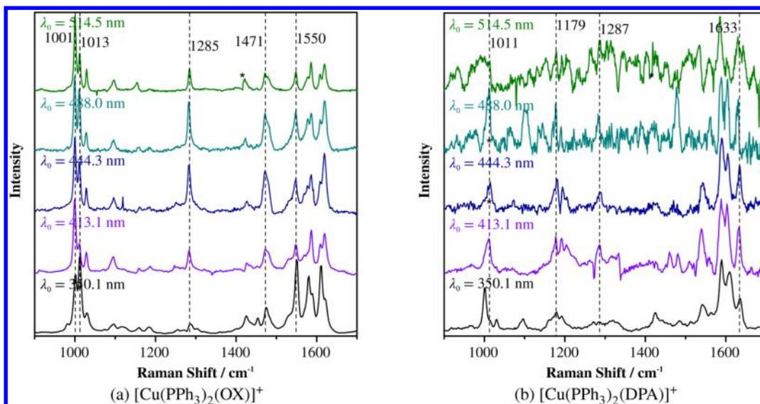
**Figure 10.** Resonance Raman spectra at various excitation wavelengths, acquired in  $\text{CH}_2\text{Cl}_2$ : (a)  $[\text{Cu}(\text{PPh}_3)_2(\text{OX})]^+$  and (b)  $[\text{Cu}(\text{PPh}_3)_2(\text{DPA})]^+$ . Solvent subtraction has been performed. Residuals that appear are marked with asterisks.
