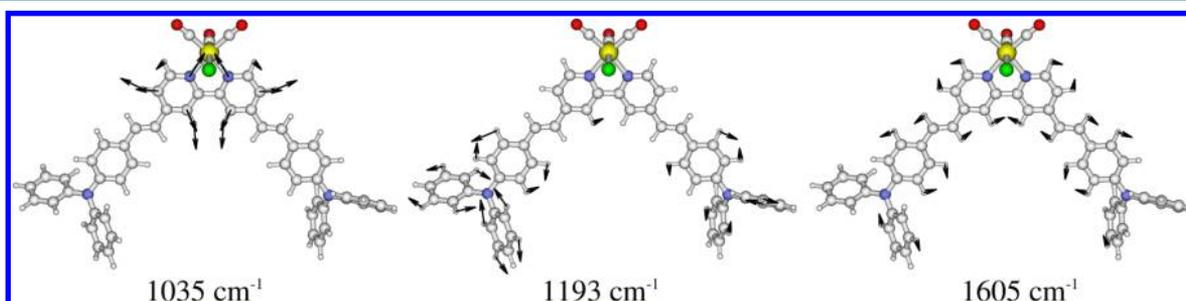
**Figure 9.** Examples of normal modes, with their corresponding *calculated* wavenumbers, corresponding to bpy-centered, diphenylamine-centered, and delocalized vibrations seen in the resonance Raman spectra of  $[\text{Re}(\text{CO})_3\text{Cl}(\text{DPA})]^+$ .
