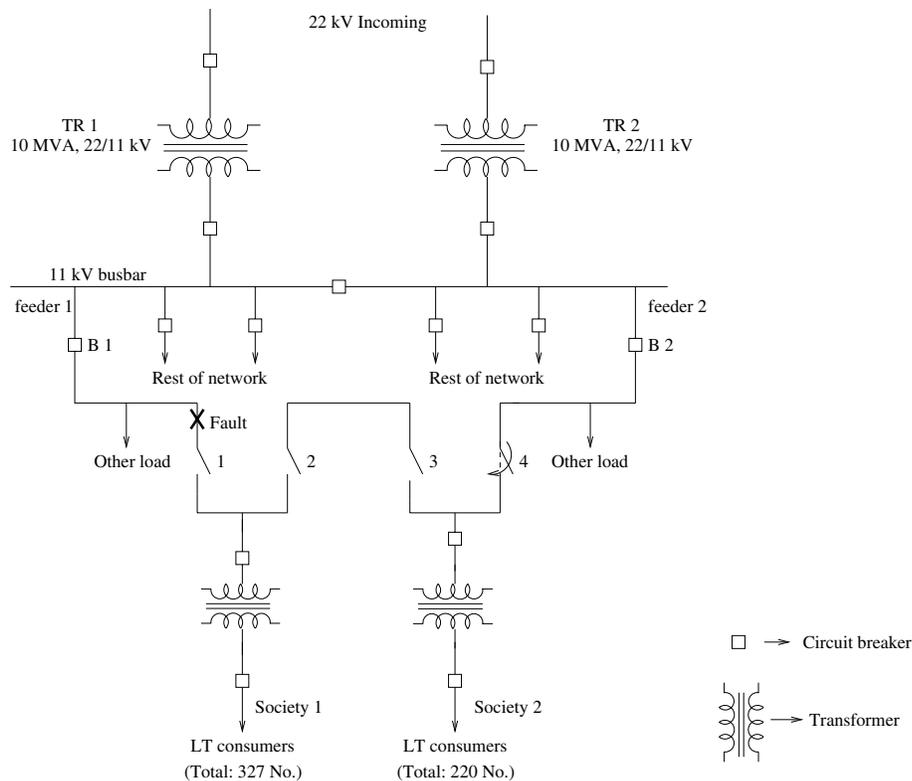
Fig. 4 Practical distribution system with fault on feeder 1
