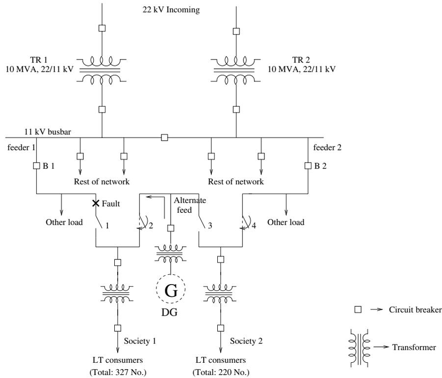
Fig. 5 Inclusion of DG for supplying isolated load
