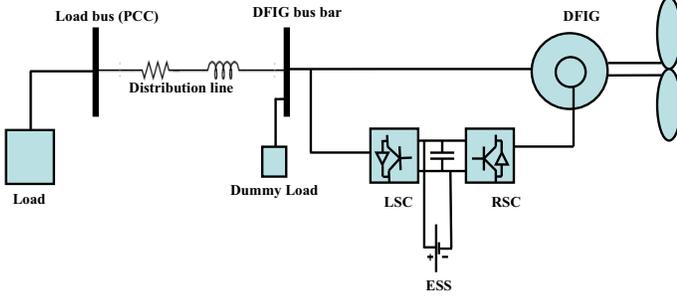
Fig. 1. Proposed Remote Area Power System
