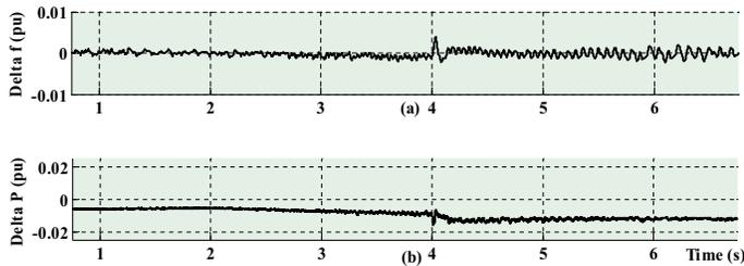
Fig. 12. Frequency and Power Deviation of the System (a) Frequency Deviation and (b) Active Power Imbalance
