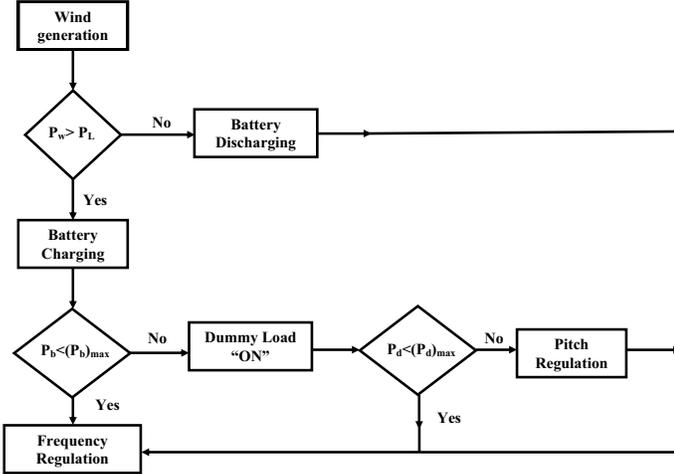
Fig. 7. Control Coordination of Proposed RAPS System
