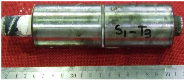
Fig.3 - Failure along the bolt grout interface in push test at 150 mm encapsulation length
