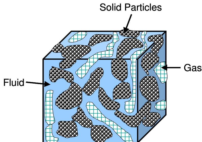
Figure 4.1 An illustration of three phases of porous media
