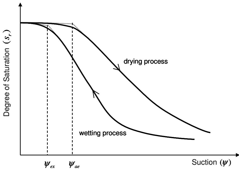
Figure 4.2 Schematic soil water characteristic curve
