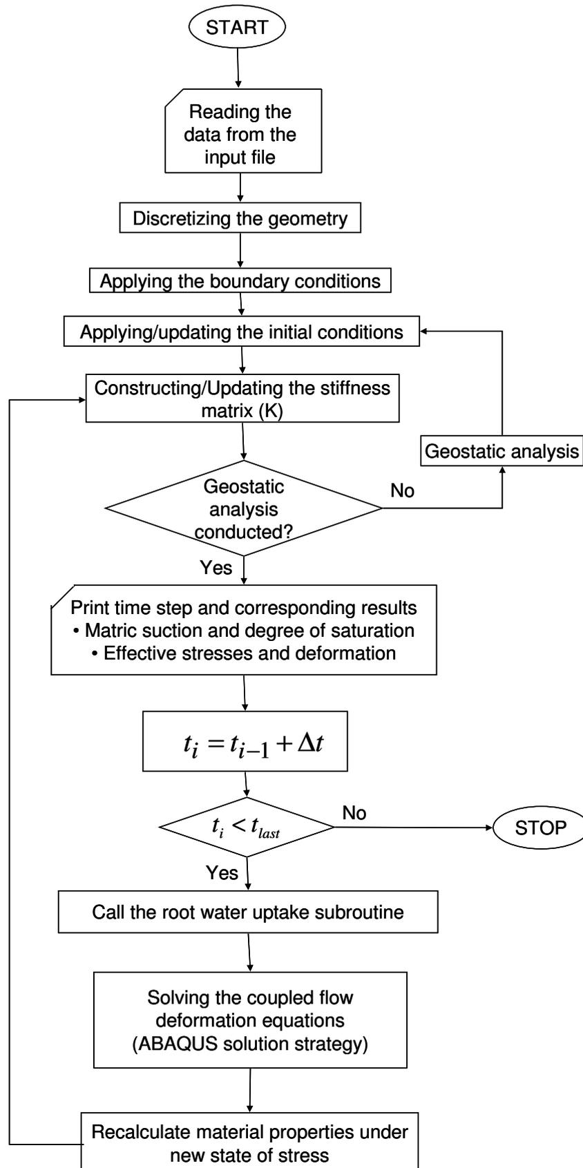
Figure 4.3 Flow chart of approximate solution of coupled-flow deformation governing equation
