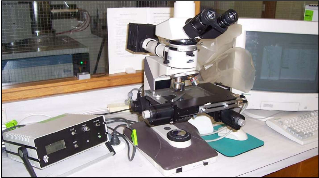
Figure 3.1 – Polarising microscope with Micro-GIS system to locate heavy mineral grains in the polished thin section.
