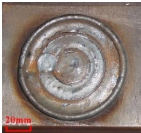
Figure 1.15: Photograph of a layer of a solid cylinder
