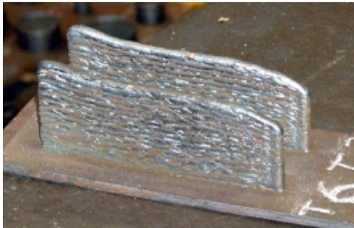
Figure 1.19: Rapid prototyped thin metal walls showing irregular geometry and
