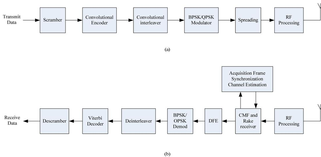
**Figure 2. Block diagram of the DS-UWB transceiver. (a) transmitter. (b) receiver.**
