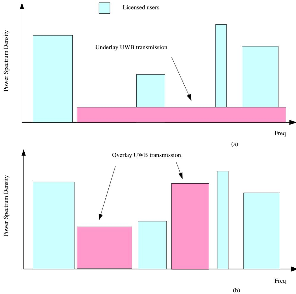
**Figure 5. (a) Underlay mode and (b) overlay mode of UWB spectrum sharing with primary users.**
