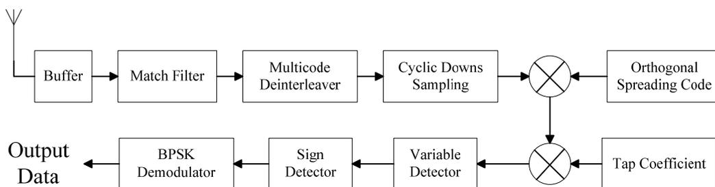
Figure 23. The DBDS receiver structure.
