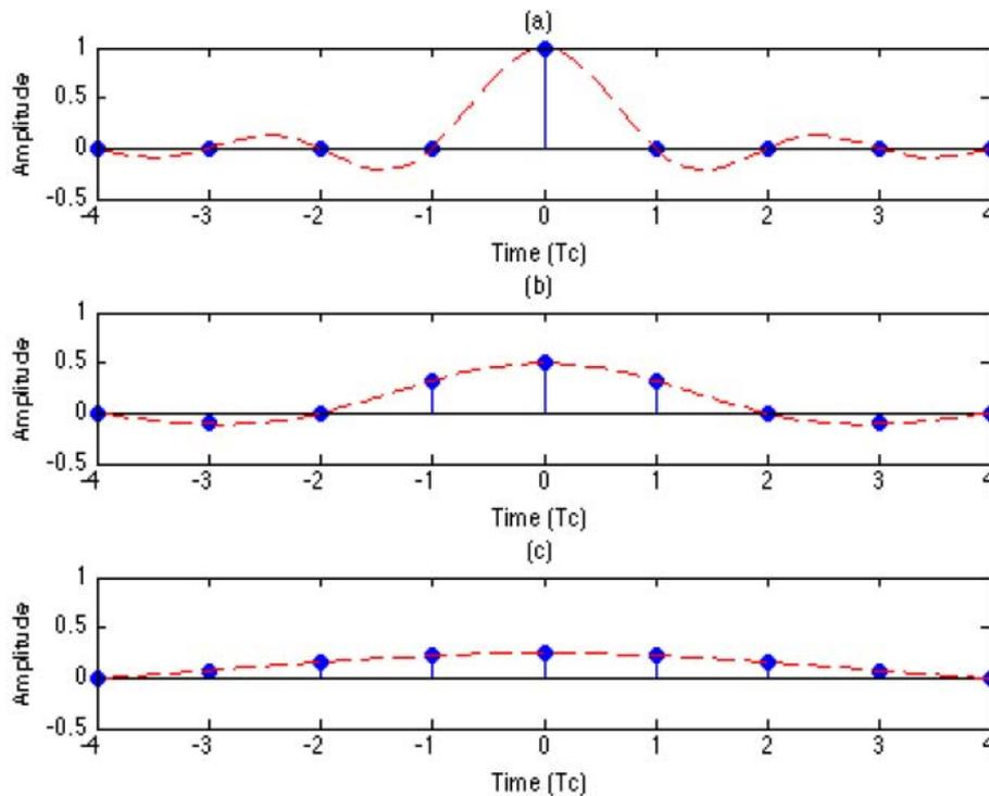
**Figure 8. Example of filtered impulses, (a)  $m = 0$ , with full bandwidth, (b)  $m = 1$ , impulse with half bandwidth (c)  $m = 2$ , impulse with quarter bandwidth.**
