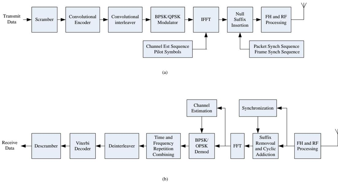
**Figure 4. Block diagram of the MD-OFDM transceiver, (a) transmitter. (b) receiver.**
