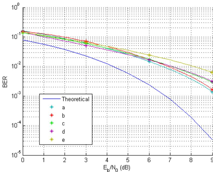
Figure 28. Average performance with (a). 1/2 band low pass filter in 2 paths channel; (b). 1/4 band low pass filter in 4 path channel; (c). 1/4 high pass filter in 3 path channel; (d). 1/4 high pass filter in 4 path channel; (e). 1/4 band pass filter in 4 path channel.
