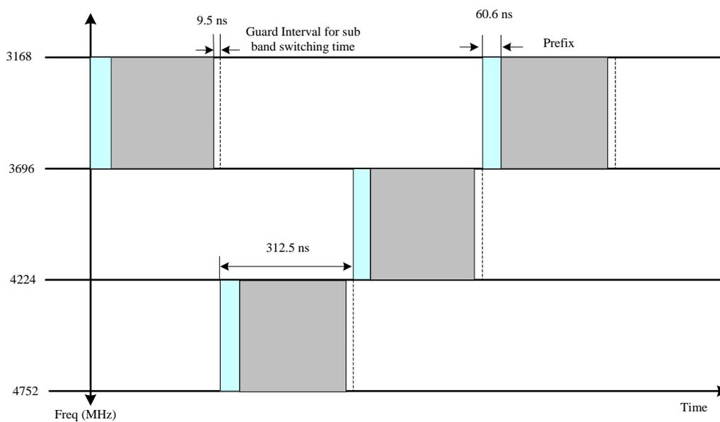
Figure 3. Example of TF coding for an MB-OFDM system [9].
