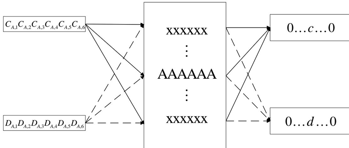
**Figure 14. Example of despreading two bits ( $c$  and  $d$ ) from the same bits (AAAAAA) using different code.**
