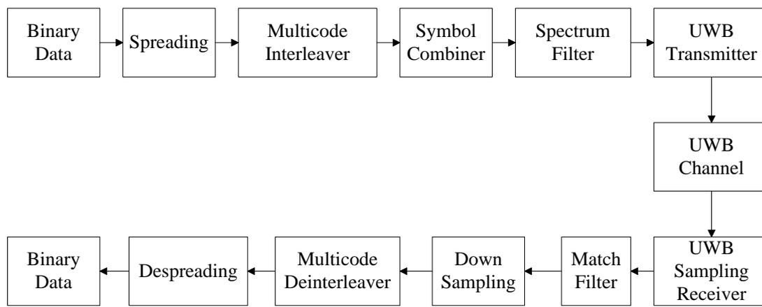
**Figure 10. Block diagram of equivalent system model.**
