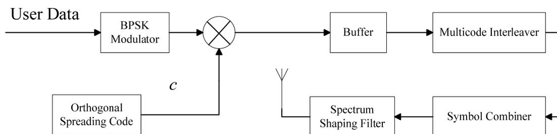
Figure 22. The DBDS transmitter structure.
