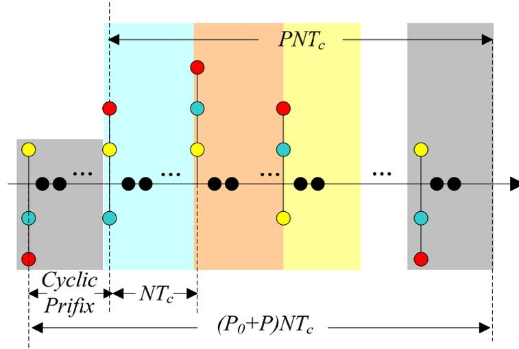
Figure 13. Every  $2^m$  chips are added into one chip, while others are set to zero.
