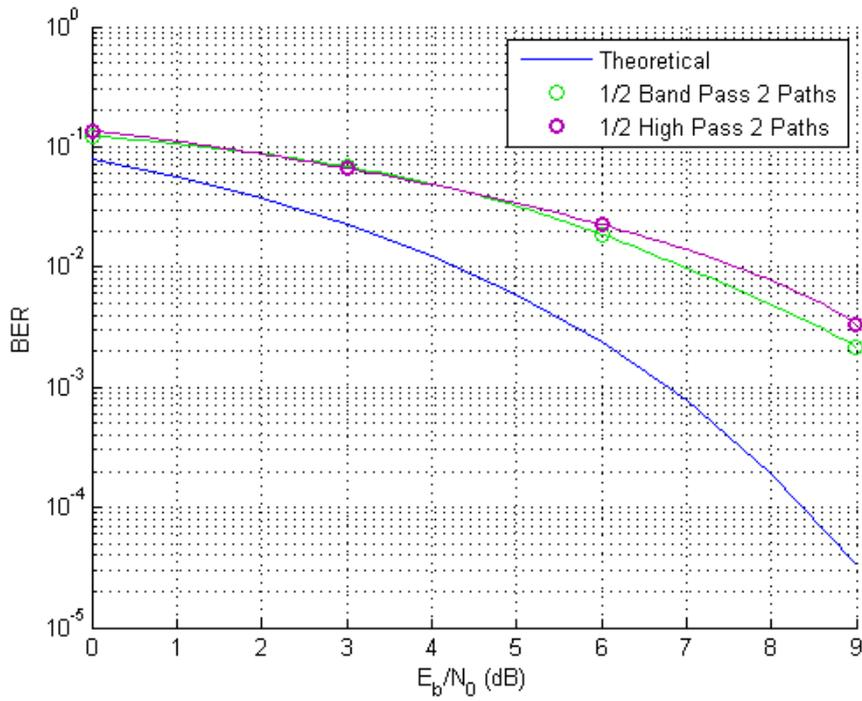
Figure 27. Average performance by half bandwidth (a) band pass and (b) high pass filter under multipath Gaussian channel.
