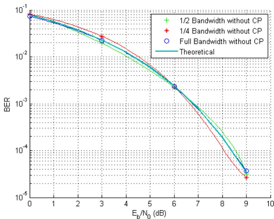
**Figure 24. Average performance for raised cosine filter under ideal Gaussian channel without CP.**
