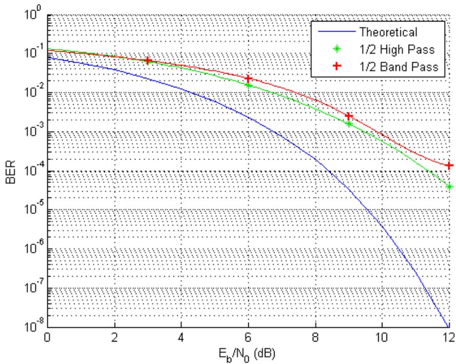
**Figure 26. Average performance using half bandwidth high pass and low pass filter with 4 bit CP in ideal Gaussian channel.**
