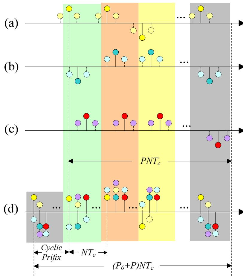
Figure 9. Spectral shaped signal sequence.
