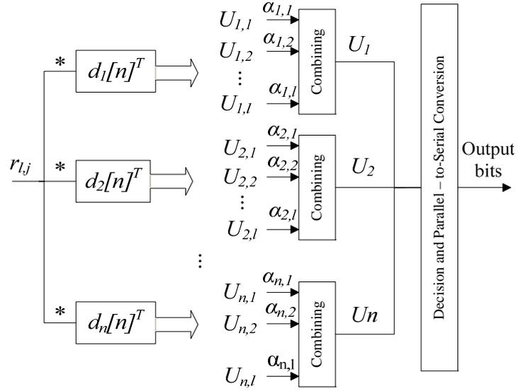
**Figure 17. Spreading and combining structure.**
