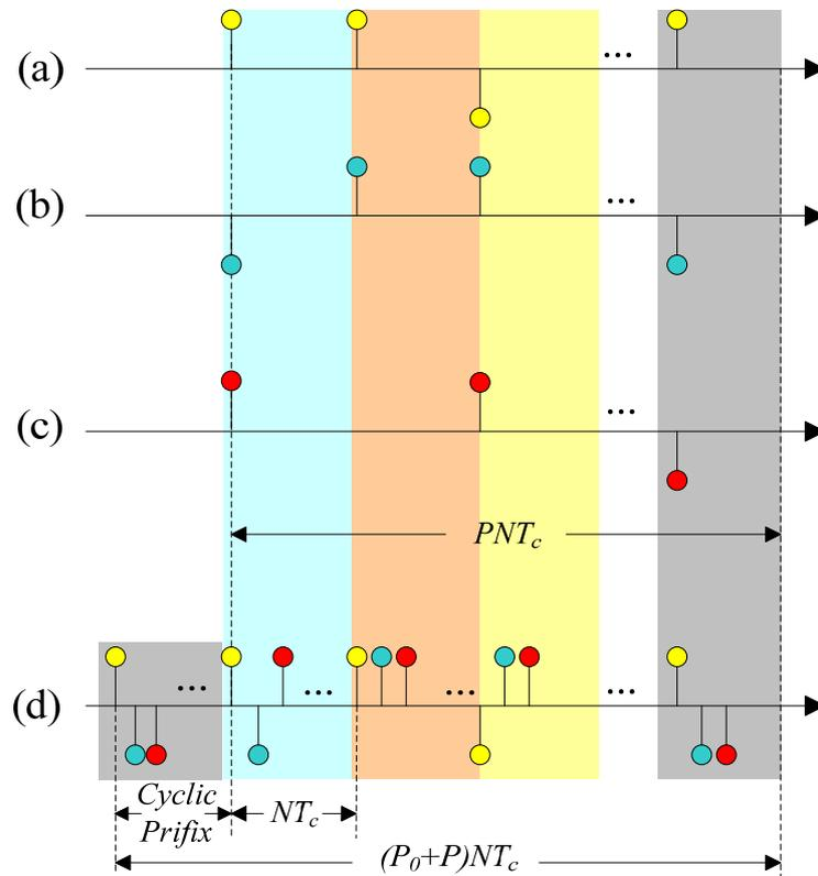
**Figure 6. An example of MCIDS spreading.**
