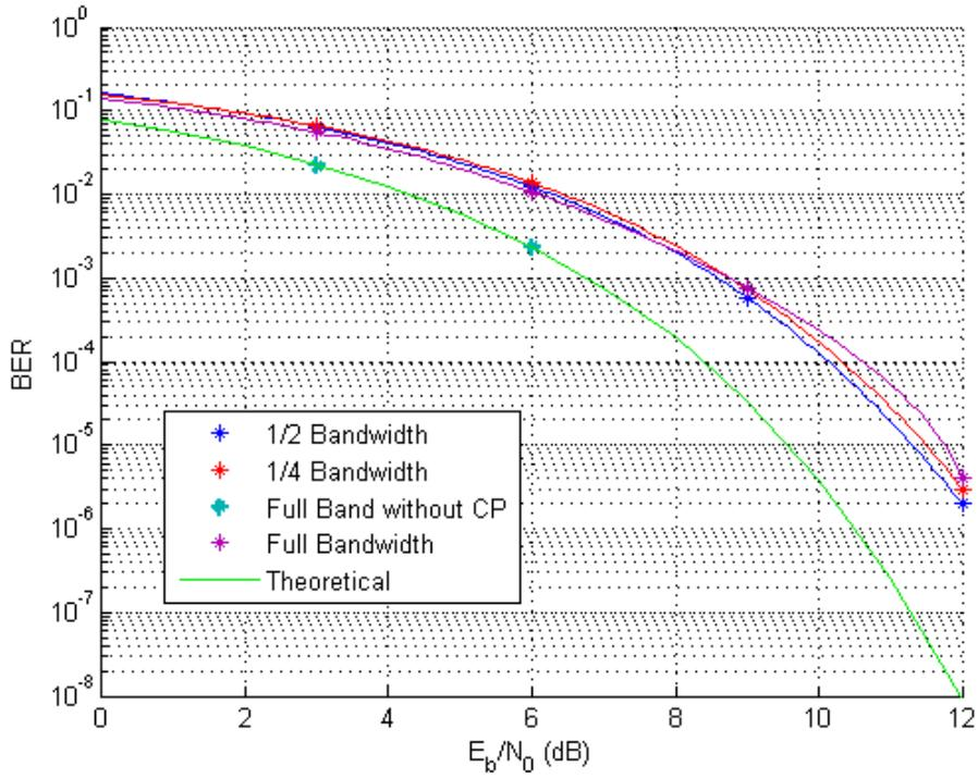
**Figure 25. Average performance using raised cosine filter with 4 bit CP in ideal Gaussian channel.**
