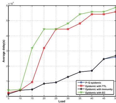
Fig. 8. Delay comparison of epidemic-based protocols under RWP.
