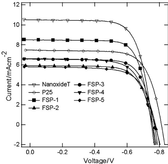
Fig. 7.  $I-V$  characteristics of DSSCs under one-sun conditions. Thickness of the TiO<sub>2</sub> electrodes was 5–6  $\mu$ m.
