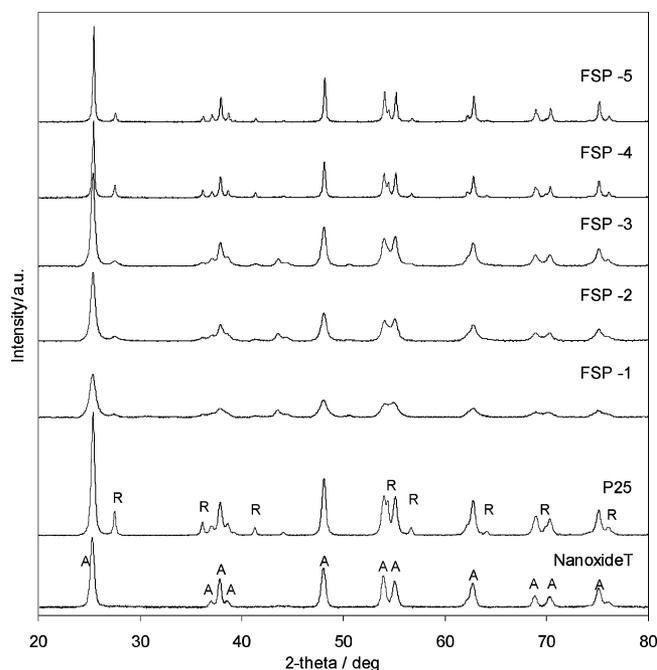
Fig. 1. XRD spectra of As-prepared FSP TiO<sub>2</sub> powder samples as well as Degussa P25 and Nanoxide-T. The characteristics peaks of anatase are labeled “A”, while those of rutile are labeled “R”.
