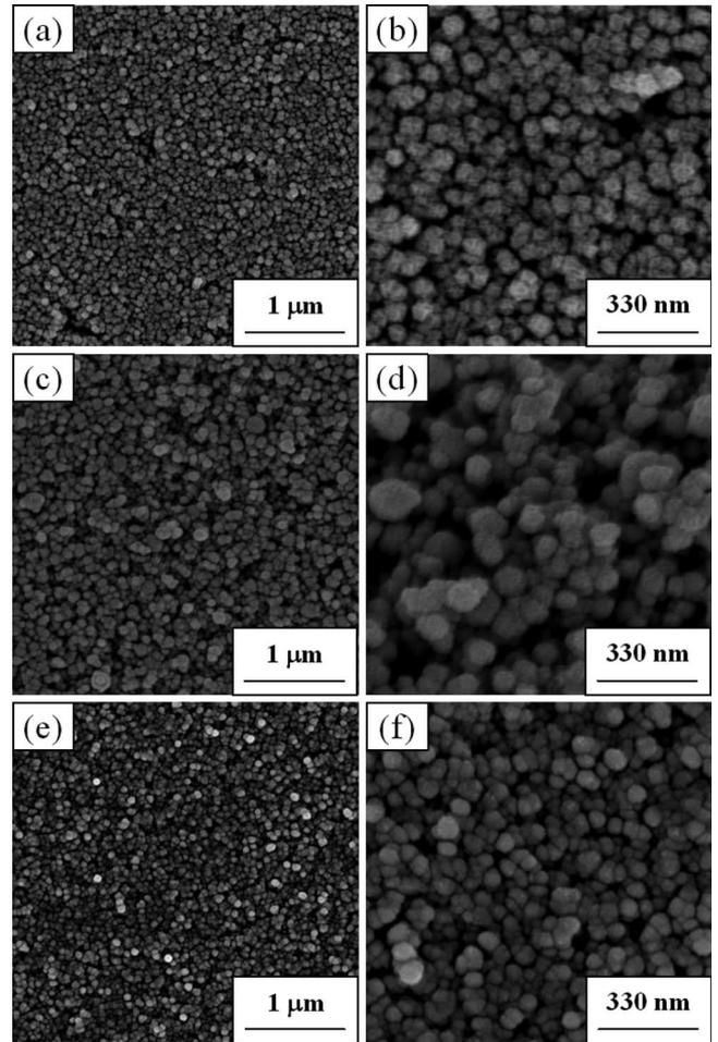
Fig. 4. SEM images of doctor-bladed  $\text{TiO}_2$  films prepared from (a) and (b) FSP-3, (c) and (d) FSP-5, and (e) and (f) commercial benchmark Nanoxide-T.
