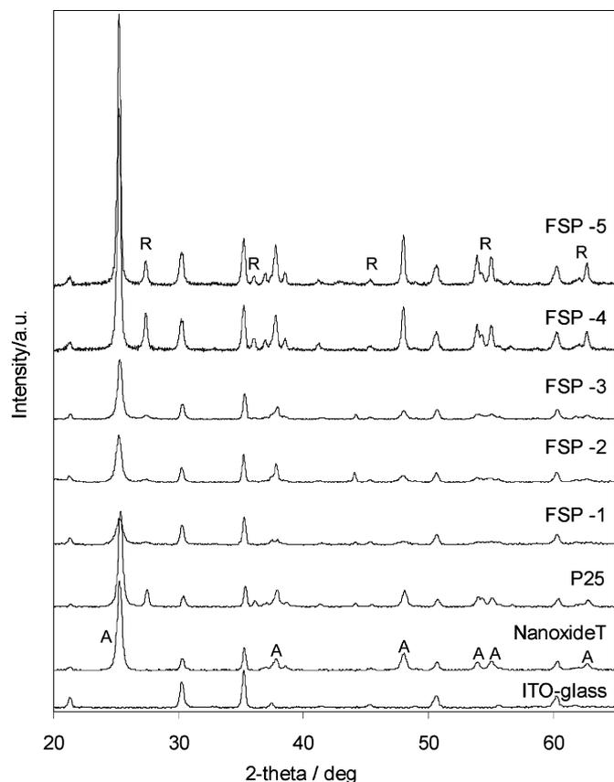
Fig. 5. XRD spectra of doctor-bladed  $\text{TiO}_2$  particulate films on conductive indium tin oxide glass, fabricated from FSP samples, as well as Degussa P25 and Nanoxide-T. The characteristics peaks of anatase are labeled “A,” while those of rutile are labeled “R.”
