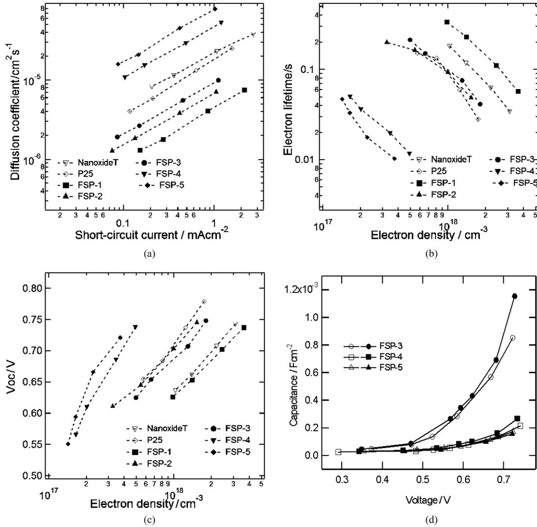
Fig. 6. (a) Electron diffusion coefficient ( $D$ ), (b) electron lifetime ( $\tau$ ), (c) open-circuit voltage ( $V_{oc}$ ), and (d) capacitance ( $C$ ) of DSSCs. For (d), data from two identical samples are shown.
