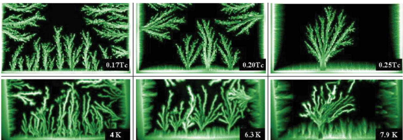
FIG. 7. (Color online) Temperature variation in the morphology of flux dendrites. Top panels show simulated results for  $B_z$ , and bottom panels show magneto-optical images of a  $\text{MgB}_2$  film.
