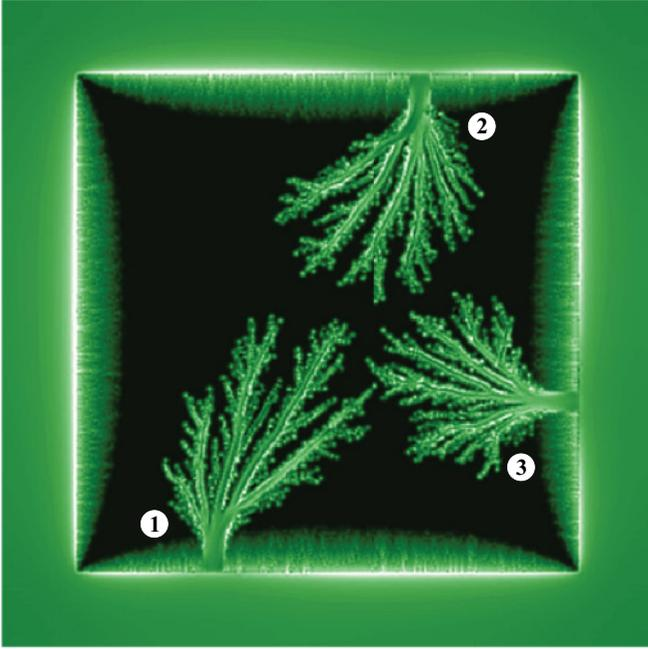
FIG. 2. (Color online) Calculated distribution of  $B_z$  at an applied field  $H_a = 0.18J_{c0}$  and substrate temperature  $T_0 = T_c/4$ . The image brightness represents the magnitude of  $B_z$ . The sample contour appears as a bright rim of enhanced field, and the black central area is the flux-free Meissner state region.
