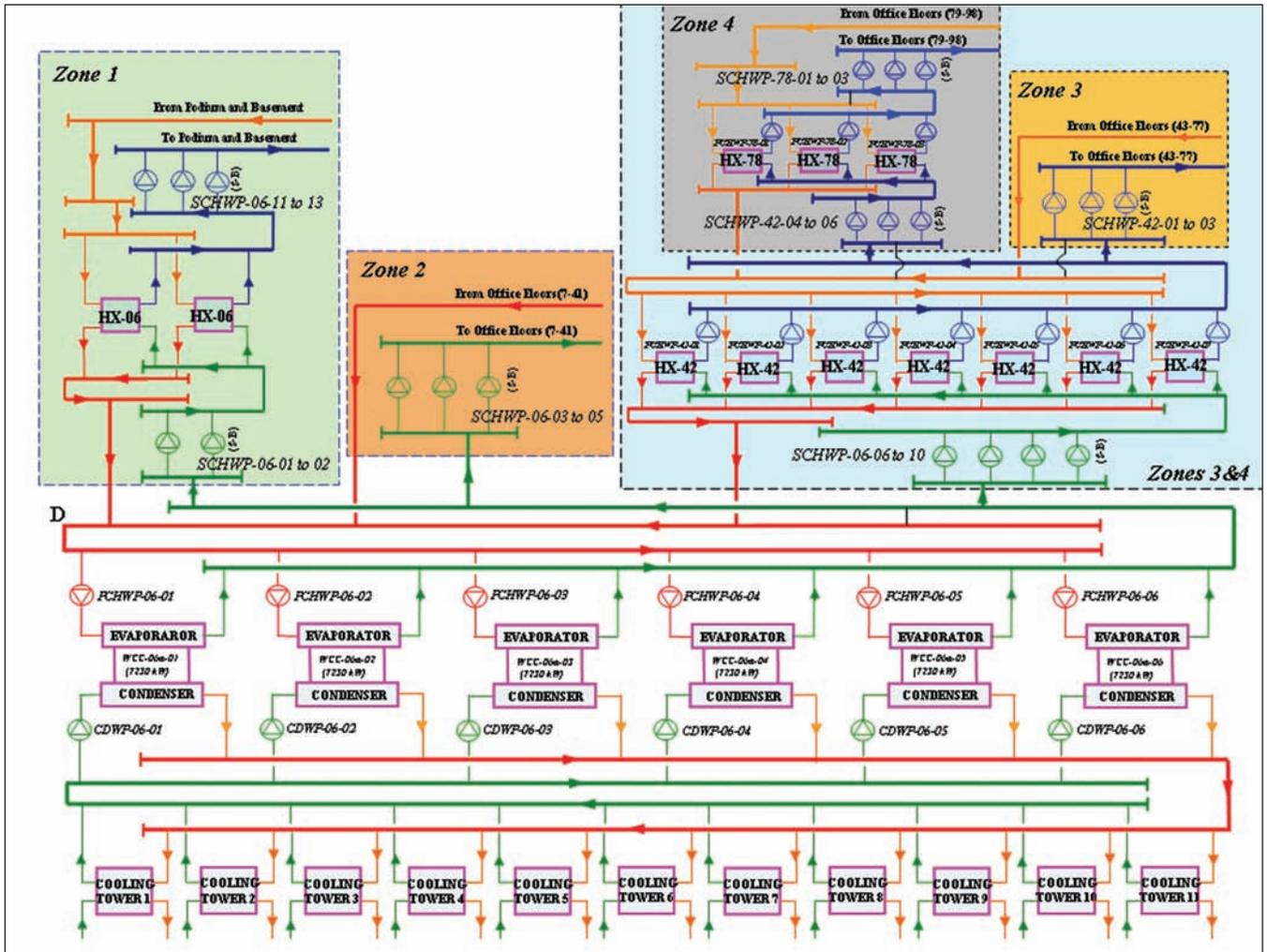
Figure 1: Schematics of the central chilling system.
