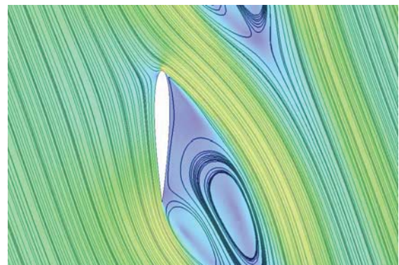
Figure 5: CFD prediction of streamlines in a tandem cascade ( \gamma = 0^\circ ) with s/c=2 and \alpha_m = 20^\circ .
