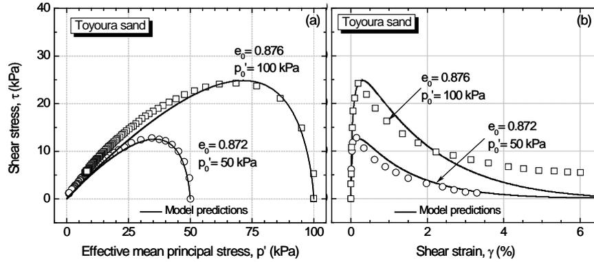
**Fig. 2.** Undrained monotonic torsional shear behavior of Toyoura sand consolidated to a void ratio  $e_0 = 0.872$ - $0.876$  (from [4]): (a) effective stress path; and (b) stress-strain relationship.
