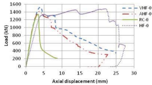
Figure 2. Load-axial deflection curves for concentrically loaded columns
