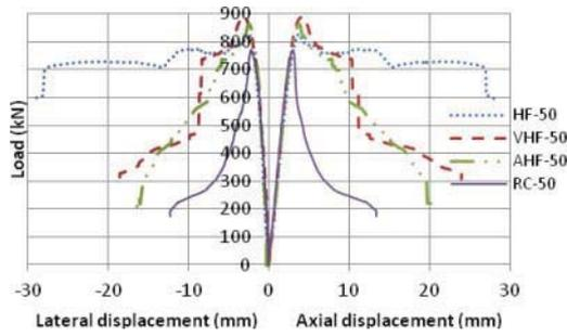
Figure 4. Load-deflection curves for 50 mm eccentrically loaded columns.
