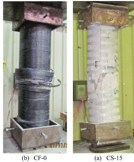
Figure 7. Failure modes of Columns CF-0 and CS-15.
