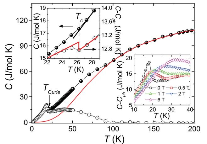
FIG. 4 (color online). Temperature dependence of specific heat before (solid symbols) and after (open symbols) deduction of lattice contribution for  $\text{EuFe}_2(\text{As}_{0.7}\text{P}_{0.3})_2$ . The solid curve represents the lattice contribution fitted by the Debye model. The upper-left panel shows the specific-heat anomaly around 26 K, which is ascribed to the superconducting transition. The lower-right panel shows the magnetic specific-heat anomaly around 20 K under magnetic fields.
