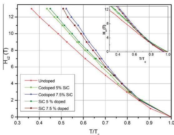
**Figure 4.** Normalized temperature dependence of the upper critical field  $H_{c2}$  for undoped, SiC-doped and co-doped  $\text{MgB}_2$  bulk samples. (Inset) Normalized temperature dependence of the irreversibility field  $H_{irr}$  of the same samples.
