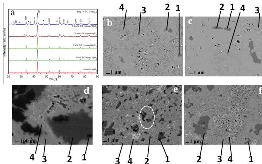
**Figure 1.** (a) X-ray diffraction patterns of the undoped, SiC-doped and co-doped  $\text{MgB}_2$  bulk samples. FESEM images of: (b) 5% SiC doped, (c) co-doped 5% SiC, (e) 7.5% SiC-doped, and (f) co-doped 7.5% SiC  $\text{MgB}_2$  bulk samples. (d) Enlarged view of the area marked in (e).
