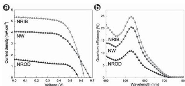
**Fig. 4** (a) Photocurrent–photovoltage characteristics and (b) incident photon to current efficiency (IPCE) of DSCs with photoanodes assembled from oriented 1D TiO<sub>2</sub> nanostructure arrays.
