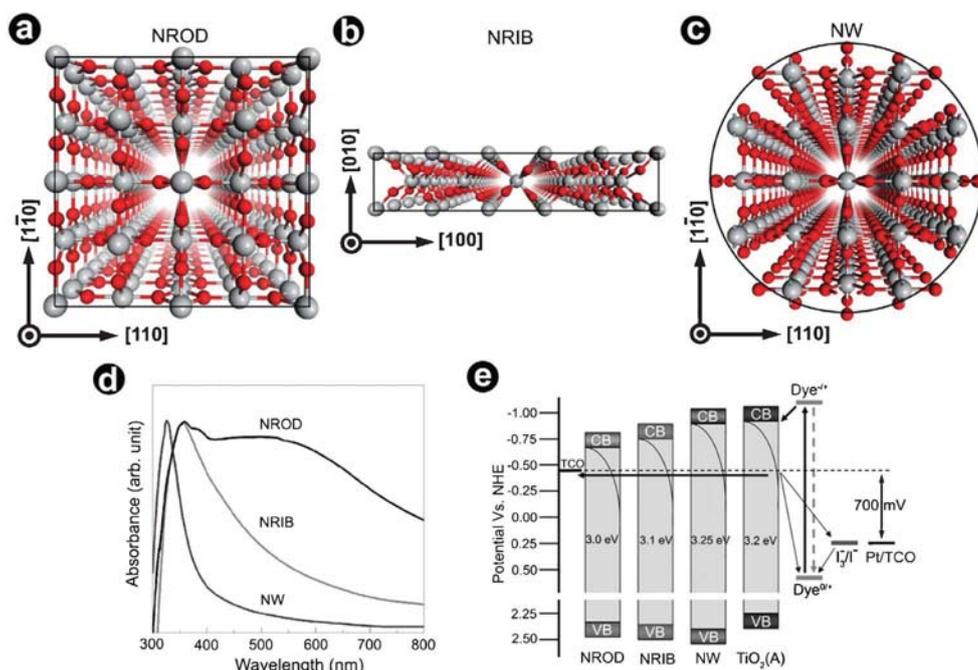
**Fig. 3** Atomic and band structures of 1D TiO<sub>2</sub> nanostructures: (a–c) diagram of atomic structure of NROD, NRIB and NW based on the TEM observation. (d) UV-Vis spectra of the NROD, NRIB and NW arrays. (e) Energy band diagrams and kinetic processes in DSCs with NROD, NRIB and NW photoanodes. As a reference, the energy level of anatase TiO<sub>2</sub> (TiO<sub>2</sub>(A)) was also incorporated.
