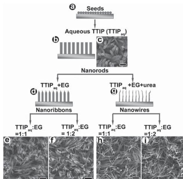
**Fig. 1** Schematic drawing and SEM images of oriented 1D TiO<sub>2</sub> nanostructure arrays synthesized under different conditions, where the morphology of 1D TiO<sub>2</sub> nanostructures changes from the form of (b–c) NRODs to (d–f) NRIBs, and then to (g–i) NWs. The scale bar in the images is 200 nm.
