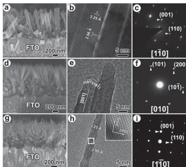
**Fig. 2** Cross-sectional SEM images, TEM images and the corresponding SAED patterns of individual 1D TiO<sub>2</sub> nanostructures: (a–c) NROD (aqueous TTIP<sub>aq</sub>), (d–f) NRIB (TTIP<sub>aq</sub> : EG = 1 : 1), and (g–i) NW (TTIP<sub>aq</sub> : EG = 1 : 2, 5 mmol urea). The inset in (h) shows an enlargement of the region indicated by the square.
