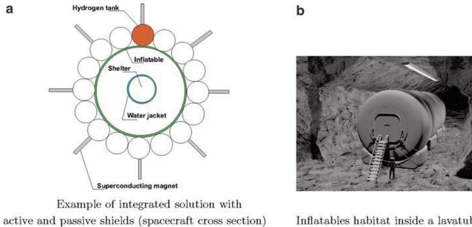
*Figure 2.* (a) Cross section of transfer vehicle, where the resources present on board are exploited for passive shielding. Liquid hydrogen tank and superconducting magnets provide a general protection against GCRs and SPEs. Drinking water stored around the crew quarters provides additional protection and shelter against strong SPEs. (b) Artistic view of an Inflatable habitat inside a lavatube on the moon (Courtesy of M. Villanti).
