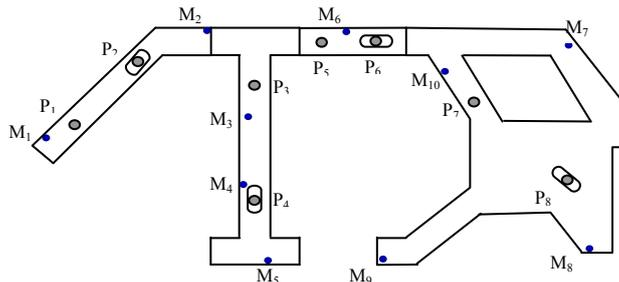
**Fig 3.** Case study: Side frame of Sports Utility Vehicle with locating pins and measurement points
