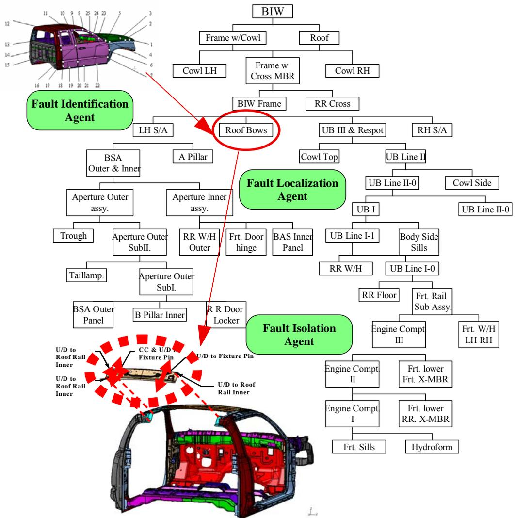
Fig. 2. Model-based diagnosis using Fault identification, localization, and isolation agents on Heirarchical Groups of autobody product
