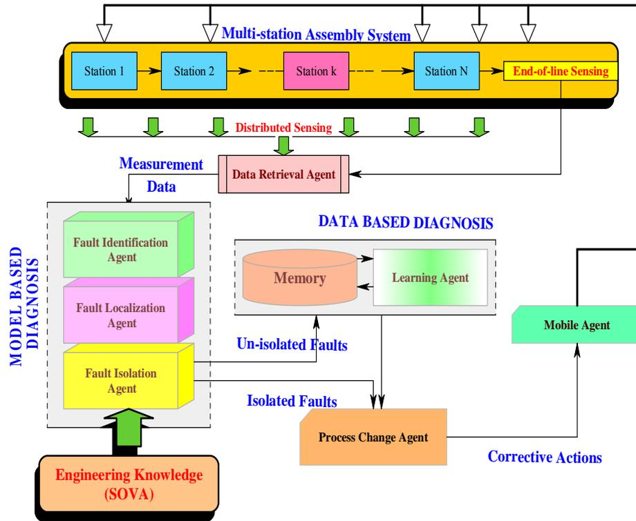
Fig. 1. ABSM architecture for fault diagnosis in Multi-station Assembly Processes.
