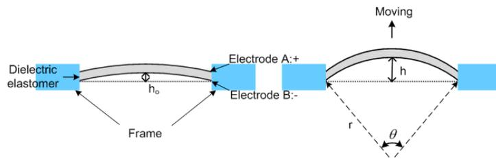
Figure 1. Working principle of tactile stimulator
