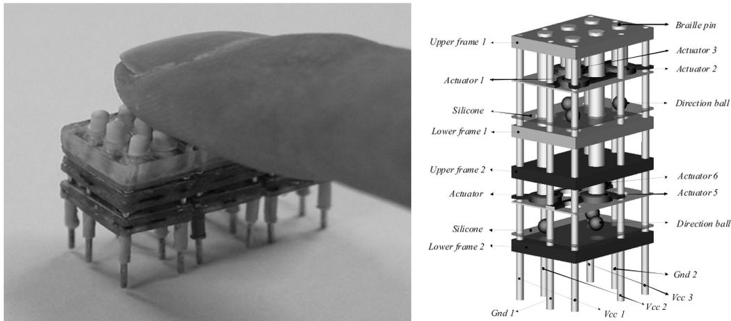
Figure 4. Dynamic Braille display and its design
