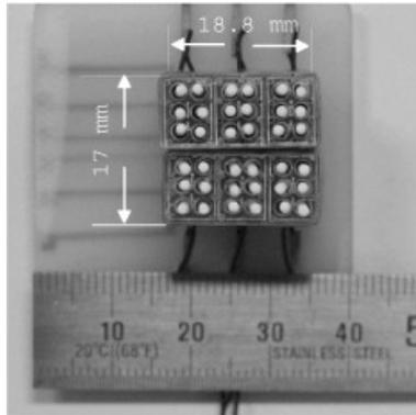
Figure 5. Braille tablet by assembling six modules of Braille cells
