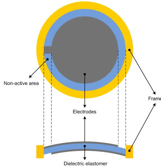
Figure 2. Construction of tactile stimulator
