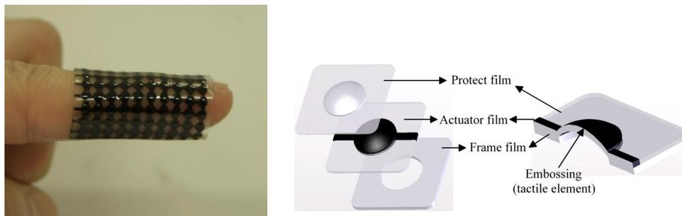
Figure 6. Wearable tactile display
