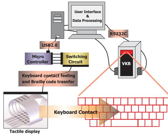
Figure 8. System layout of virtual keyboard with tactile display
