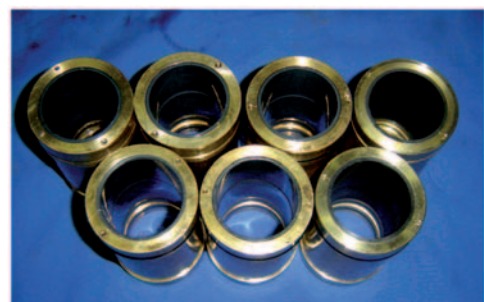
Fig. 10 Picture of sleeves with CFRP liner
