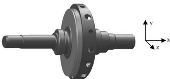
Fig. 11 Three-dimensional drawing of the unbalanced shaft assembly
