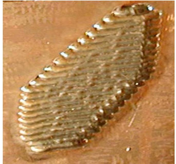
Figure 8. repair patch complete
