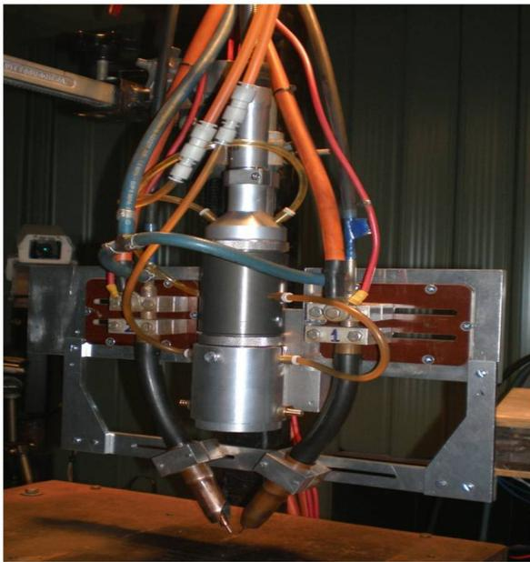
Figure 5. Prototype tandem GMAW system
