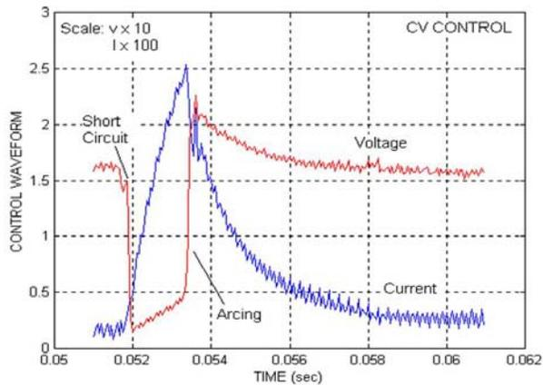
Figure 1. A single cycle of a conventional dip transfer waveform (short circuit and arcing period)
