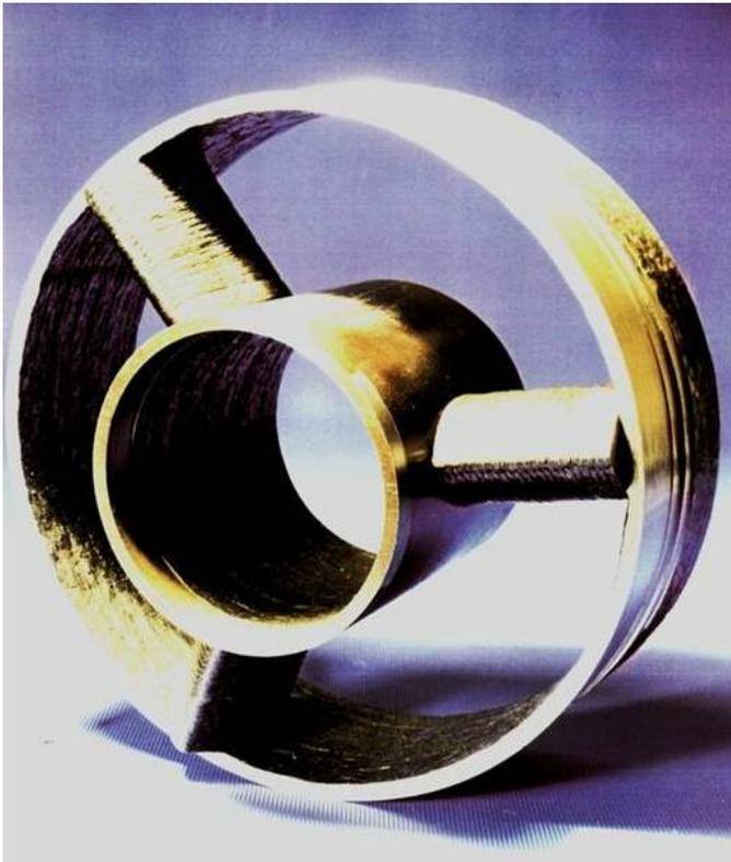
Figure 9 Complex fabrication formed by direct metal deposition
