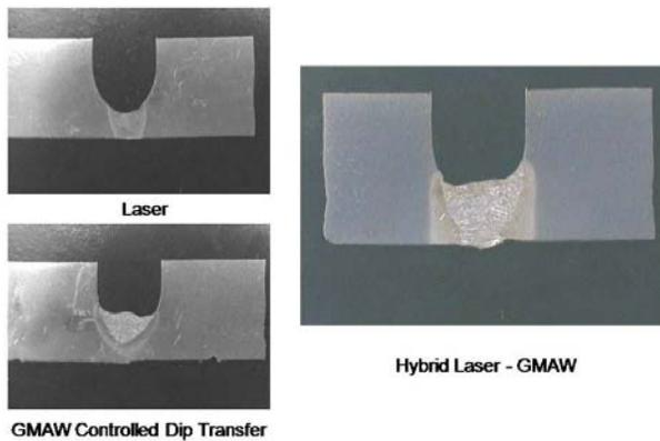
Figure 4. Comparison of root runs made in a closed J butt with a 3kw diode laser, controlled dip transfer and a hybrid combination of the 2. The material was carbon manganese steel, the root face was 1.6mm and the travel speed 1000mm/min.
