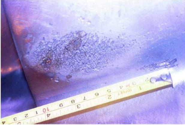
Figure 6. Cavitation damage on a hydro turbine runner
