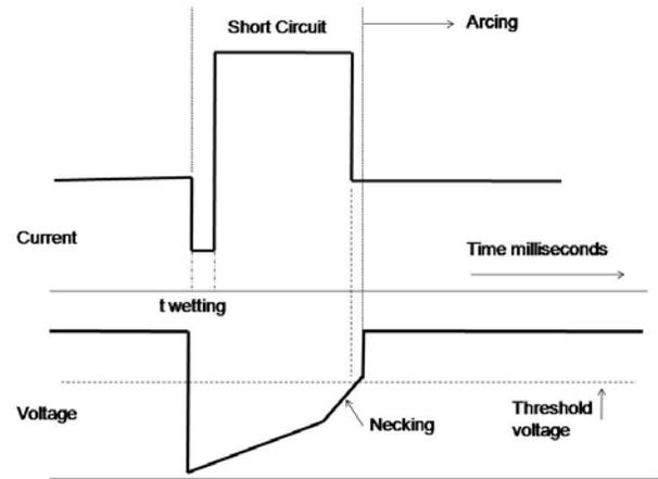
Figure 2. Diagrammatic illustration of short circuit control system devised by Boughton
