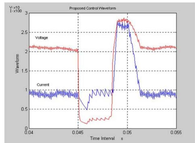
Figure 3 Simplified controlled dip transfer waveform.
