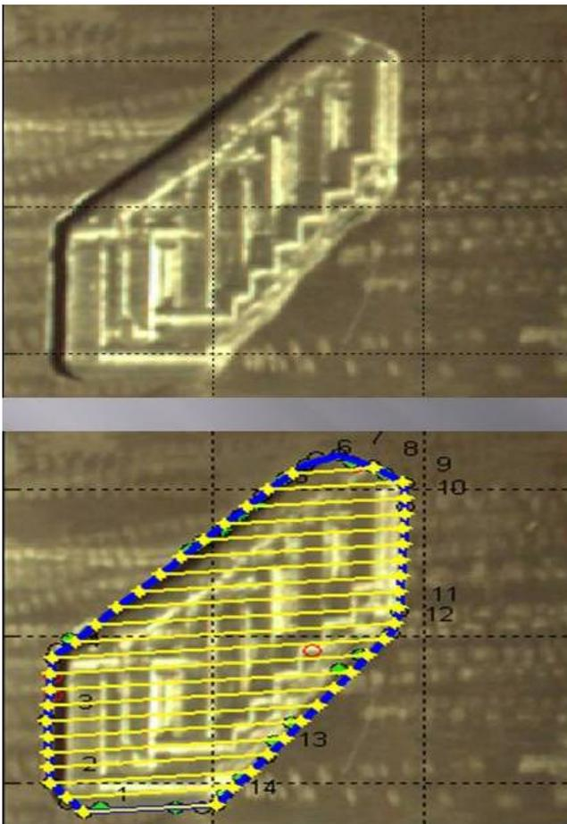
Figure 7top- a simulated wear cavity, bottom – the automatically generated weld paths.
