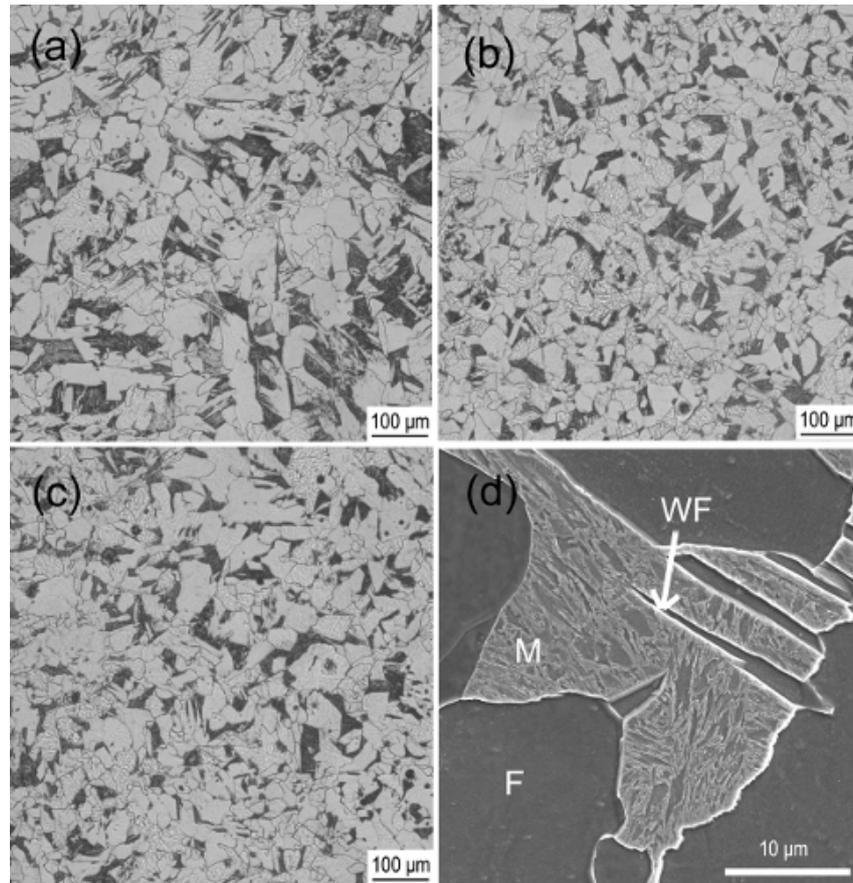
**Figure 4.** Microstructures and martensite distribution after holding at 650 °C for (a) 100 s and (c, d) 300 s, and holding at (b) 670 °C for 300s: *F* ferrite, *M* martensite, *WF* Widmanstätten ferrite.
