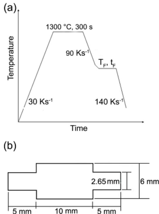
**Figure 1.** Schematic diagram of (a) heat treatment applied to the (b) samples to simulate strip casting.
