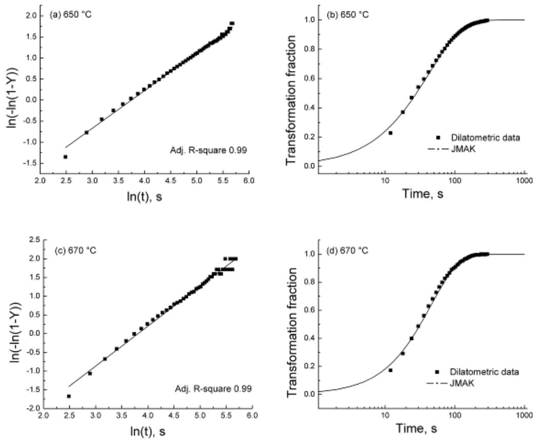
**Figure 5.**  $\ln(-\ln(1-Y))$  as a function of holding time at (a) 650 °C and (c) 670 °C; the fittings of Avrami equation at (b) 650 °C and (d) 670 °C.
