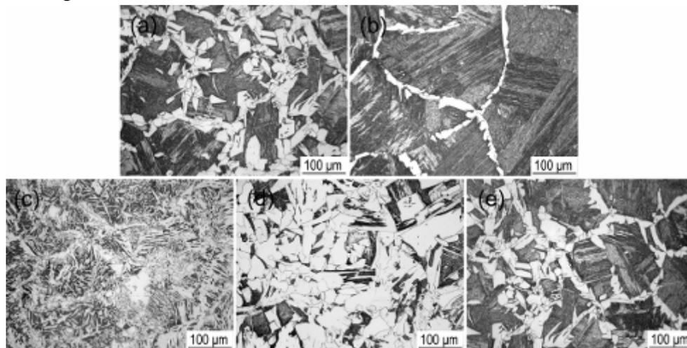
**Figure 2.** Microstructures after austenitising at 1300 °C for 180 s followed by holding at (a) 650 °C for 60 s, (b) 670 °C for 60 s, (c) 600 °C for 180 s, (d) 650 °C for 180 s and (e) 700 °C for 180 s.
