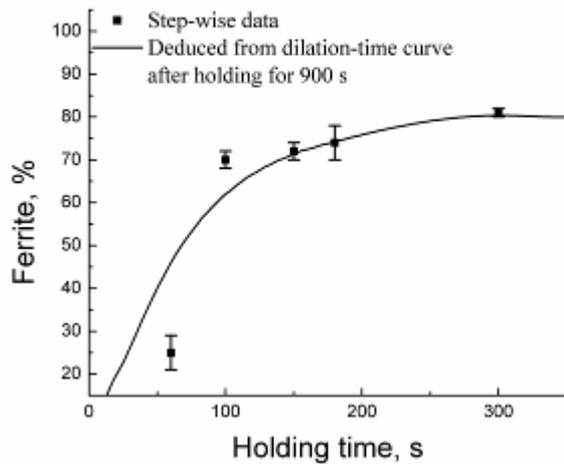
**Figure 3.** Variation in volume fraction of ferrite with time of holding at 650 °C.
