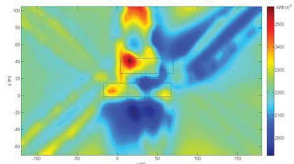
Figure 13 Annual wind energy density ( $\text{kWh/m}^2/\text{year}$ ) at 18m elevation for the SBRC site using CFD modelling and wind speed and direction statistics.
