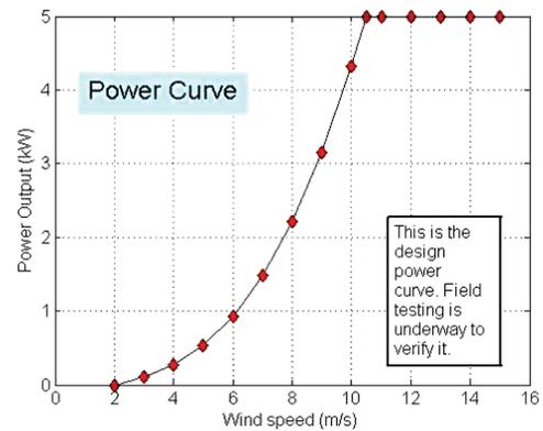
Figure 12 Aerogenesis 5kW wind turbine published power curve(Aerogenesis 2011).
