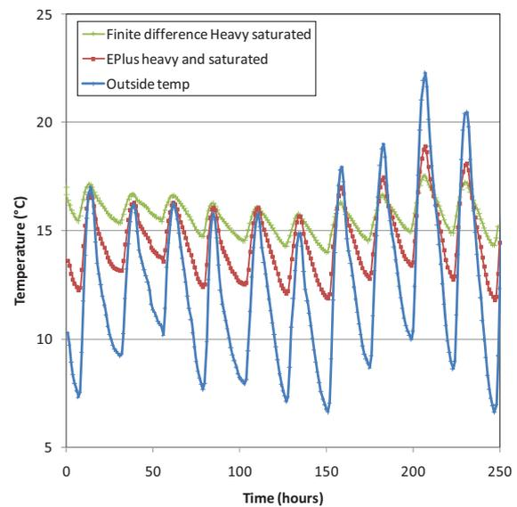
Figure 4 Simulation of air exit temperatures for a 100m-long cylindrical earth-to-air heat exchanger for typical winter conditions and assumed  $T_{soil}=18^{\circ}\text{C}$  and two different soil types.
