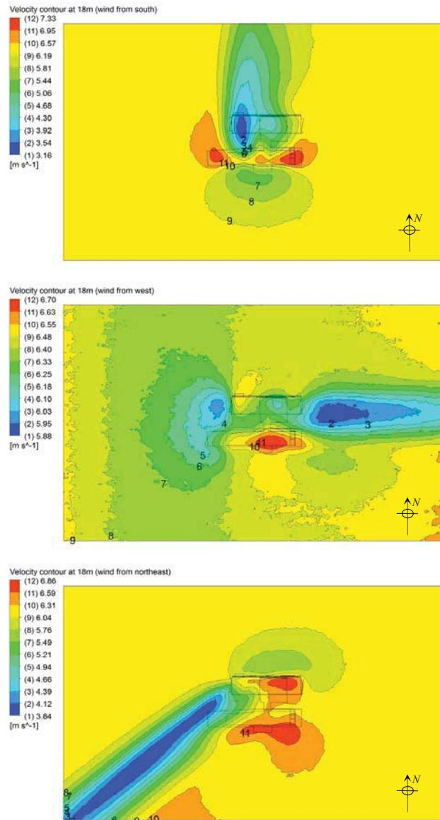
Figure 10 CFD results of wind speed at wind turbine hub elevation of 18m above ground (assuming upstream wind speed of ~6m/s at 10m).
