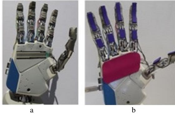
**Fig. 3.** EH1 robotic hand showing: (a) fitted force sensors and (b) neoprene covering.
