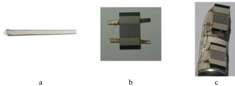
**Fig. 2.** (a). FSR480 force sensor strip. (b). Force sensor cut from FSR480 strip. (c). Cut force sensors mounted on a robotic finger.
