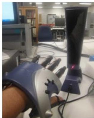
**Fig. 7.** P5 data glove for controlling the robotic hand.
