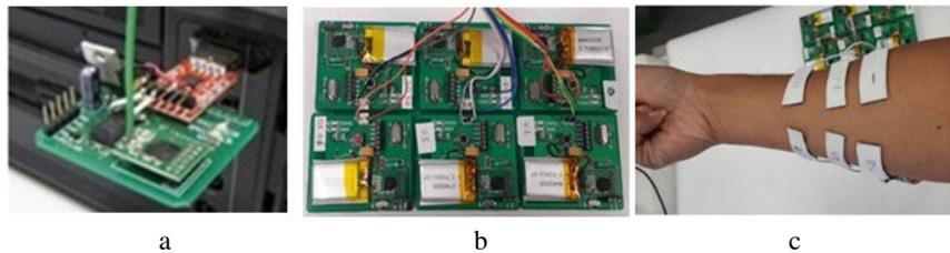
**Fig. 4.** TENS feedback System: (a) Transmitter (b) Receivers (c) Arm with electrodes fitted.
