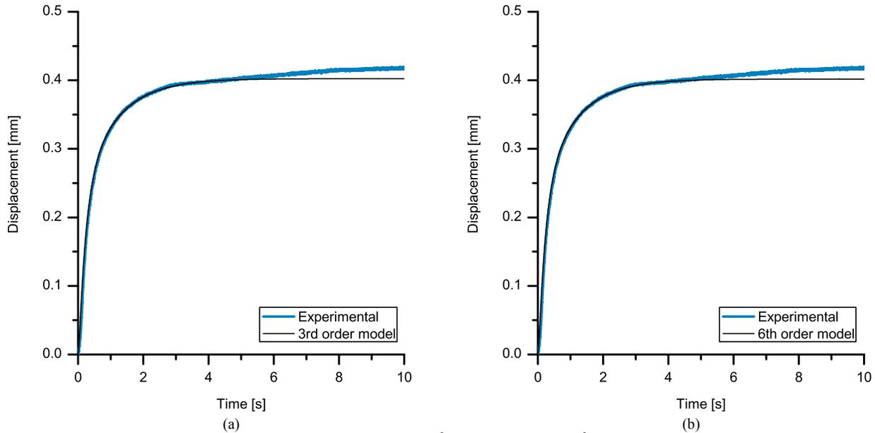
**Fig. 7: Experimentally observed and simulated (a) 3<sup>rd</sup> order and (b) 6<sup>th</sup> order step responses for a 50mV step voltage, applied to a 10mm long, 2mm wide trilayer actuator.**
