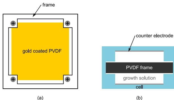
Fig. 2: Schematic of (a) PVDF stretching frame and (b) top view of the polymerization cell
