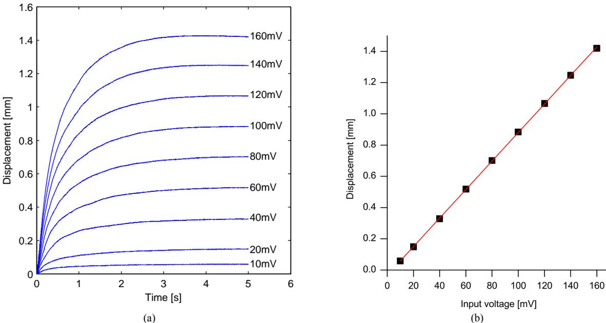
**Fig. 3: (a) Displacement response of a trilayer actuator in response to increasing amplitude step voltages, and (b) displacement at 5 seconds as a function of input voltage. A linear trendline has been fitted to (b) with the equation  $y = 0.0091x + 0.032$ .**
