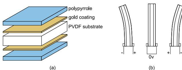
Fig. 1: (a) exploded structure and (b) bending behavior for the polypyrrole trilayer used in this study
