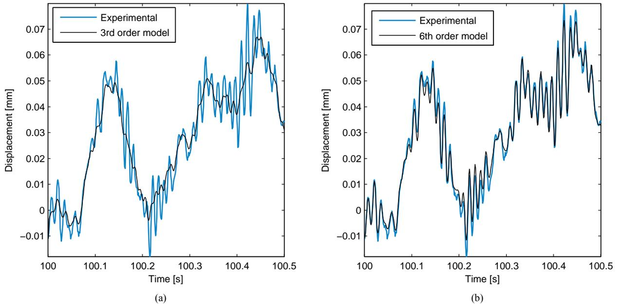
**Fig. 6: Experimentally observed response of a 10mm long, 2mm wide trilayer actuator to a random input voltage and simulated displacement from (a) a 3<sup>rd</sup> order and (b) a 6<sup>th</sup> order fitted transfer function.**
