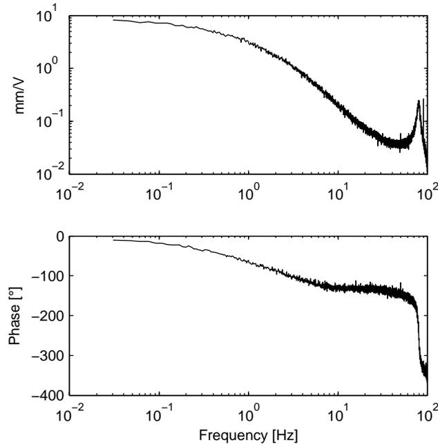
**Fig. 4: Example frequency response for a 10mm long, 2mm wide actuator**
