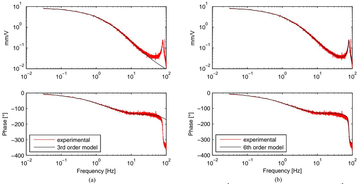
**Fig. 5: Experimentally identified frequency response and fitted (a) 3<sup>rd</sup> order transfer function and (b) 6<sup>th</sup> order transfer function**
