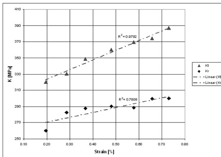
Fig. 6. Variation of stiffness coefficients vs. input isometric strain.
