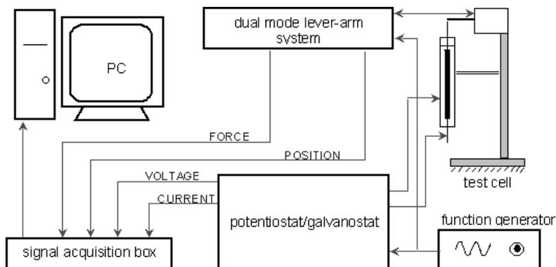
Fig. 4. Instruments configuration.
