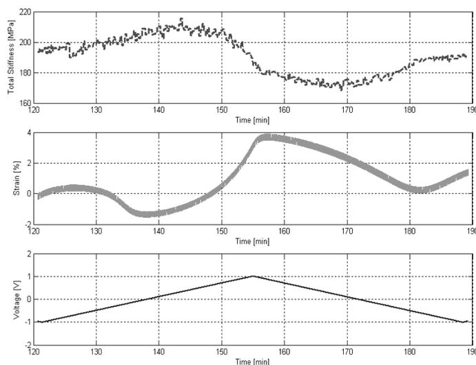
Fig. 10. Effect of actuation on total stiffness coefficient.
