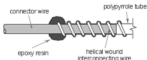
Fig. 1. Structure of PPy helix tube actuator.
