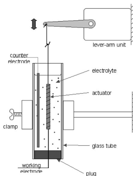
Fig. 2. Installation of actuator.
