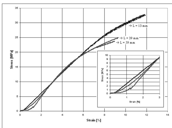
Fig. 7. Stress-strain curves for different length of actuator.
