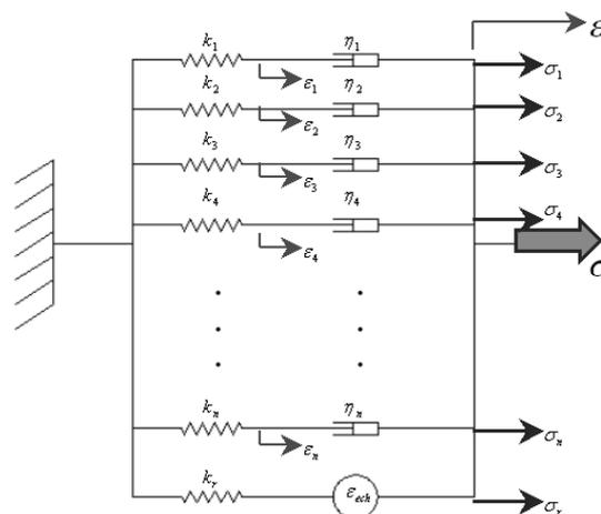
Fig. 5. Viscoelastic model of the actuator.
