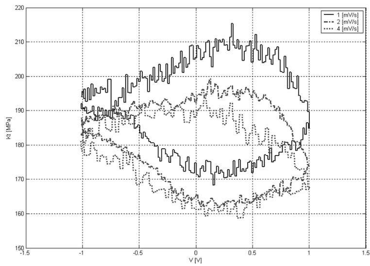
Fig. 12. Stiffness variation during actuation in different scan rates.
