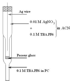
Fig. 3. Ag/Ag+ Reference electrode.
