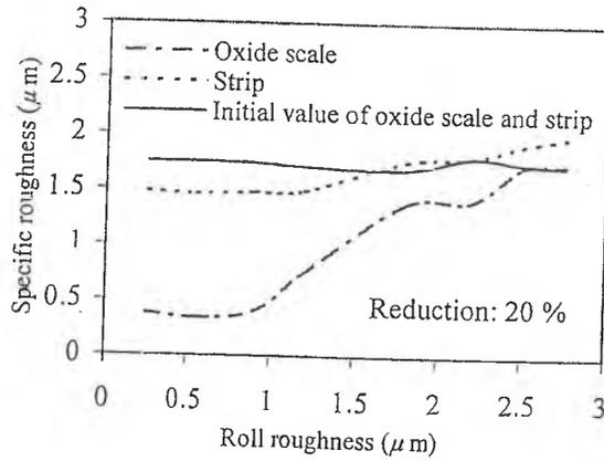
Fig. 6 Effect of the work roll surface roughness on the specific surface roughness
