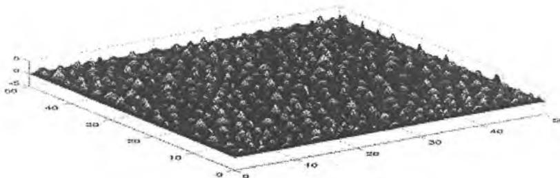
Fig. 2 A generated random surface roughness
