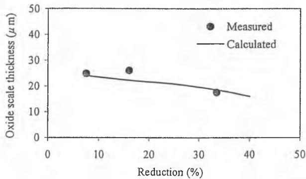
Fig. 5 Effect of reduction on oxide scale thickness
