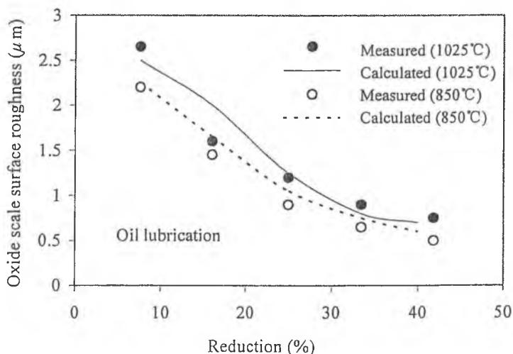
Fig. 9 Effect of rolling temperature on oxide scale surface roughness
