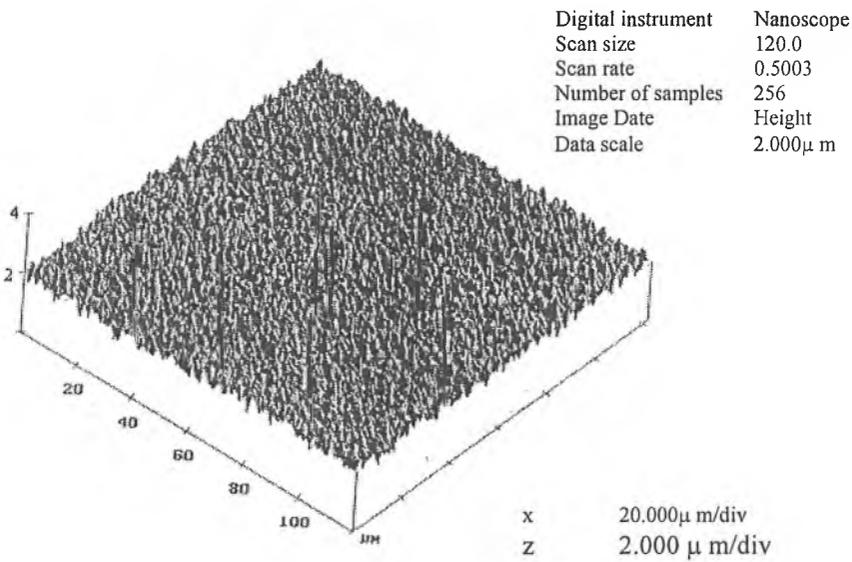
Fig. 1 3D surface image of oxide scale scanned by atomic force microscope
