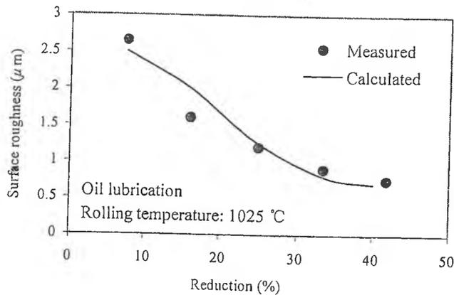
Fig. 8 Effect of reduction on surface roughness with oil lubrication
