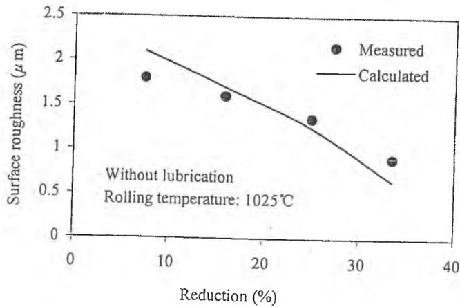
Fig. 7 Effect of reduction on surface roughness
