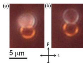
**Fig. 8** Polarization microscope images of a colloidal particle with an attached nematic LC droplet observed in reflected light enlarged to show the “on-off” effect (see text) before (a on) and during (b off) hopping of the particle along a BW.
