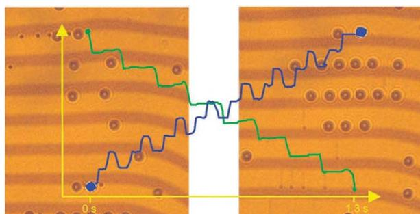
**Fig. 5** Polarization microscope images separated by a time interval of 1.3 s of a small (green) and large (blue) particles subjected to a Lissajou-like magnetic modulation (see text) having  $\hat{H} = 8500 \text{ A m}^{-1}$  and frequency  $\Omega = 18.8 \text{ s}^{-1}$ . The tracked trajectories of the small (green) and large (blue) particles are superimposed to the images. The movie (video 4) in the ESI† shows the particle separation above the magnetic stripe pattern.
