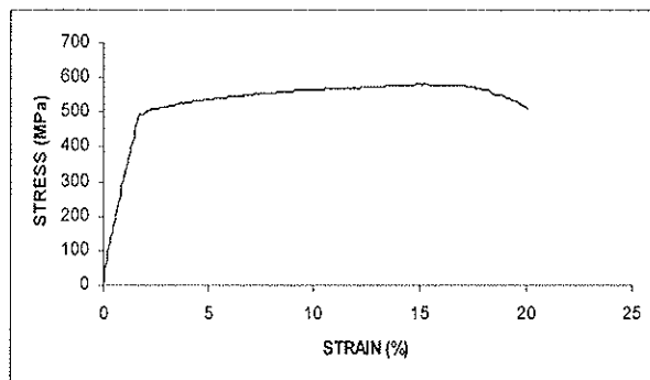
Fig. (2). Tensile stress strain curve for helical steel with 8 mm diameter.
