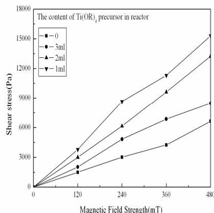
**Figure 4.** Effects of the TiO<sub>2</sub> contents on MR properties of the Fe<sub>3</sub>O<sub>4</sub>-TiO<sub>2</sub> nanocomposites based MR fluids.
