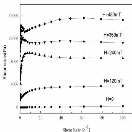
**Figure 3.** Influence of shear rate on shear stress for Fe<sub>3</sub>O<sub>4</sub>-TiO<sub>2</sub> nanocomposites based MR fluids under various magnetic fields
