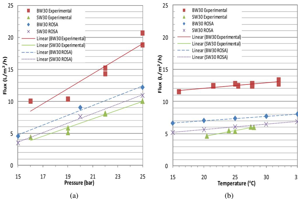
**Figure 3** (a) Experimental and simulated membrane flux as a function of pressure ( $T=25\text{ }^{\circ}\text{C}$ ,  $\text{pH}=7$  and  $\text{TDS feed}=18,000\text{ppm}$ ); (b) Experimental and membrane flux as a function of temperature ( $P=18\text{ bar}$ ,  $\text{pH}=7$  and  $\text{TDS feed}=18,000\text{ppm}$ )
