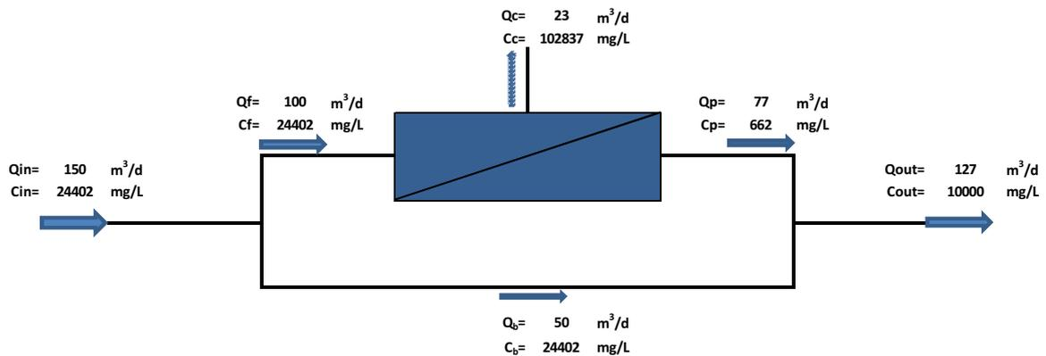
**Figure 4** Mass balanced low TDS RO system with bypass/permeate blending
