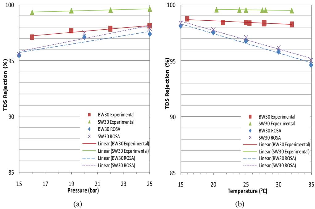
**Figure 2** (a) Experimental and simulated TDS rejection as a function of pressure ( $T=25\text{ }^{\circ}\text{C}$ ,  $\text{pH}=7$  and  $\text{TDS feed}=18,000\text{ppm}$ ); (b) Experimental and simulated TDS rejection as a function of temperature ( $P=18\text{ bar}$ ,  $\text{pH}=7$  and  $\text{TDS feed}=18,000\text{ppm}$ )
