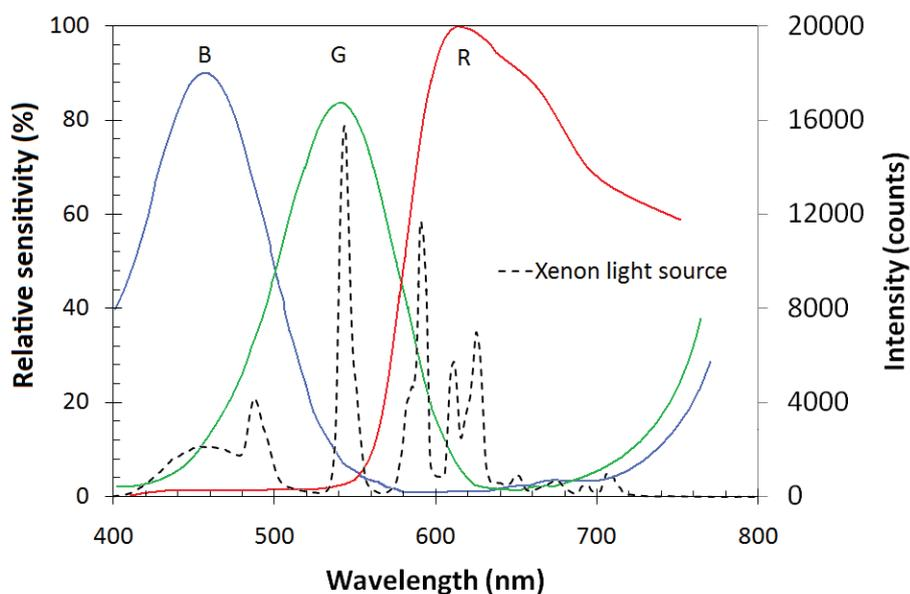
**FIGURE 10:** Typical spectral sensitivities of the red, green and blue channels of a CCD of the type used in flatbed scanners, also shown is the emission spectrum of the Xenon cold cathode ray tube used in the EPSON 10000XL flatbed scanner.
