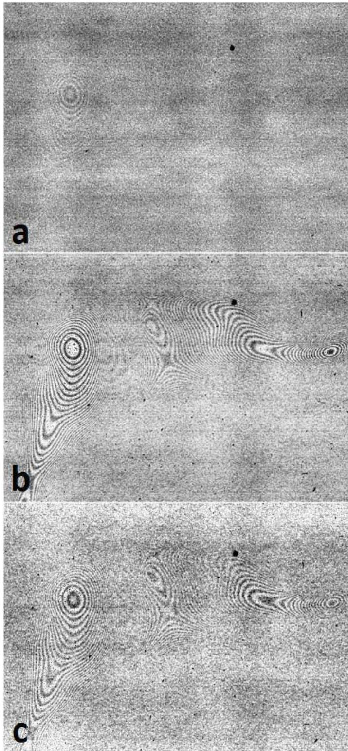
**FIGURE 11:** Interference patterns known as Newton's rings occur due to the multiple reflections at the interface between the film and glass plate of the flatbed scanner. These images are of GAFchromic<sup>TM</sup> EBT2 film and show the difference in appearance of the rings when analyzing the (a) blue, (b) green and (c) red channel data.
