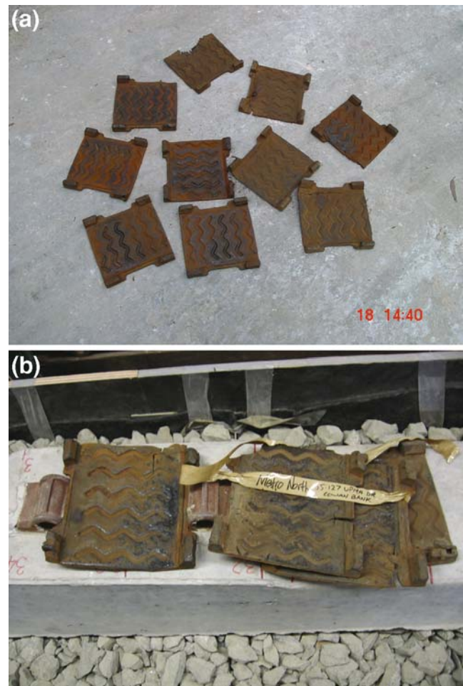
Fig. 7 Worn rail pads (a) after 99 MGT in service on RailCorp track, (b) after 110 MGT in service on RailCorp track
