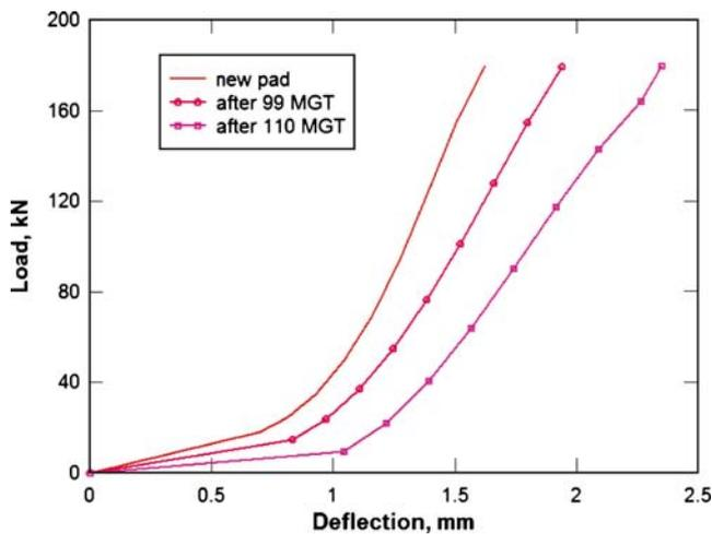
Fig. 8 Load–deflection curves of worn rail pads
