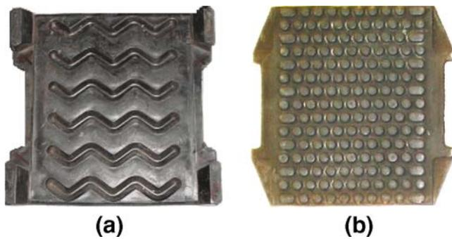
**Fig. 1** Rail pad specimens. (a) HDPE 5.5 mm (b) studded 6.5 mm
