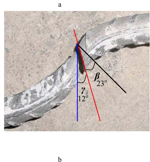
Figure 9 (a) Relationship between failure load and maximum tensile strength of the single shear on bolt type T5, (b) bolt failure angle
