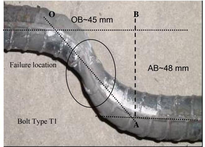
Figure 11. Excessive bolt necking in concrete 100 MPa in 80 kN pretension load, Bolt Type T1
