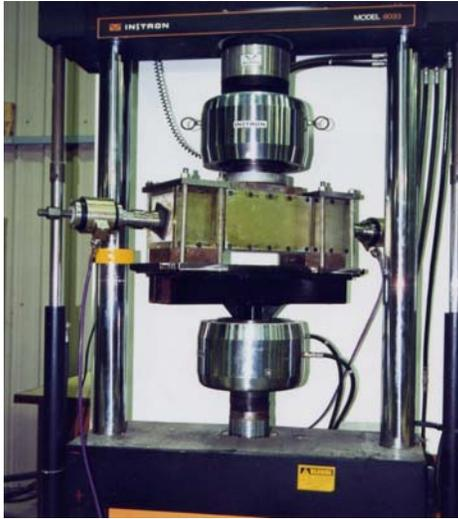
Figure 1. General set-up of the assembled double shear box unit in the testing machine
