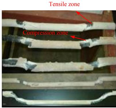
**Figure 3. Bolt deformation with tension and compression zones after the test**
