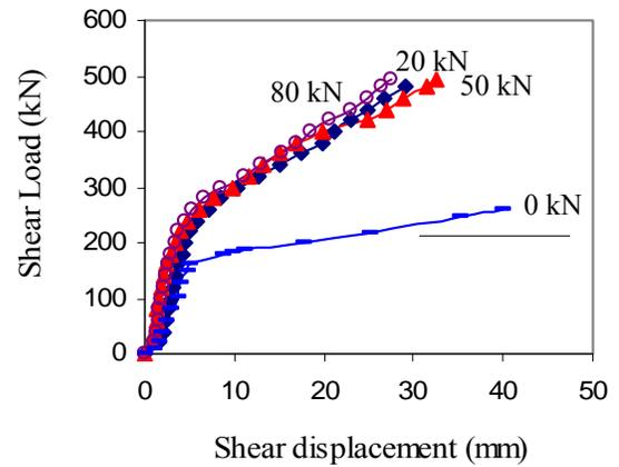
**(b) Bolt Type T2 in 40 MPa concrete**
