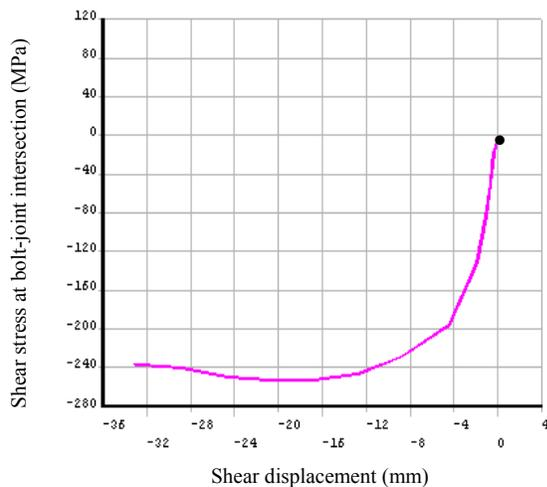
Figure 14. Shear stress trend in bolt –joint intersection in 20 MPa concrete in post failure region and 20 kN pretension load
