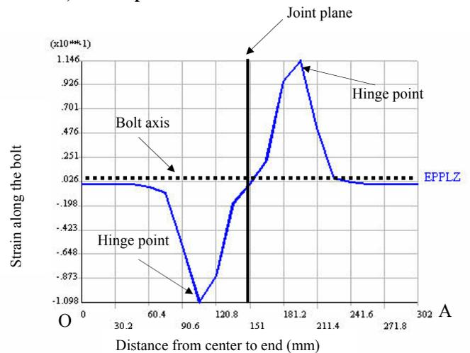
Figure 16. Plastic strain trend in 20 MPa concrete in upper fiber of the bolt without pretension load
