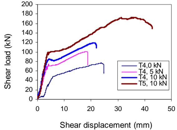
Figure 8. Shear load versus shear displacement in 0, 5 and 10 kN pretension load in Bolt Types T4 and T5 in 40 MPa concrete
