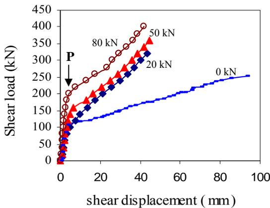
**(a) Bolt Type T1 in 20 MPa concrete**
