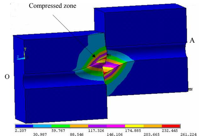
Figure 17. Yield stress induced in 20 MPa concrete without pre-tension
