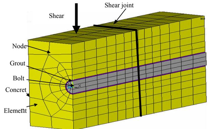
**Figure 13. Three-dimensional meshed model of a quarter section of the composite concrete/resin and bolt**
