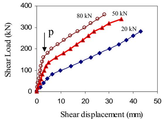
**(a) Bolt Type T3 in 20 MPa concrete**
