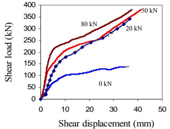
**(a) Bolt Type T2 in 20 MPa concrete**
