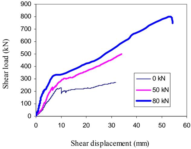
Figure 10. Shear load versus shear displacement in 100 MPa concrete and different pretensioning, Bolt Type T1
