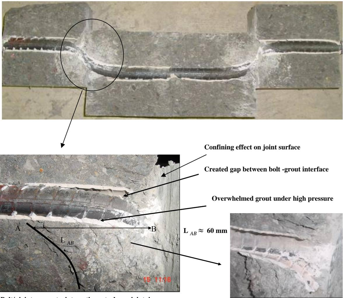
Figure 12. Bolt/ joint concrete interaction at shear joint in concrete 100 MPa and 80 kN pretension load
