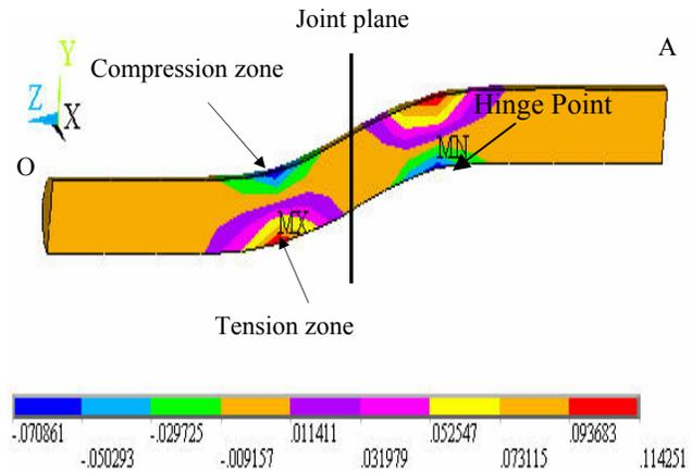
Figure 15. Plastic strain contour along the bolt axis in 20 MPa concrete, without pretension load
