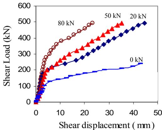
**(b) Bolt Type T1 in 40 MPa concrete**
