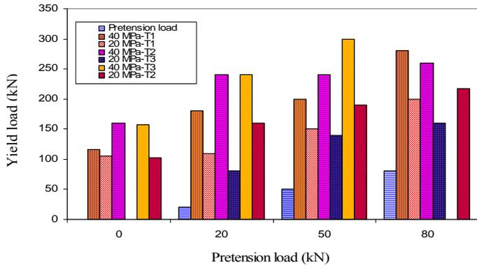
Figure 7. Comparative results in different bolt type and concrete medium
