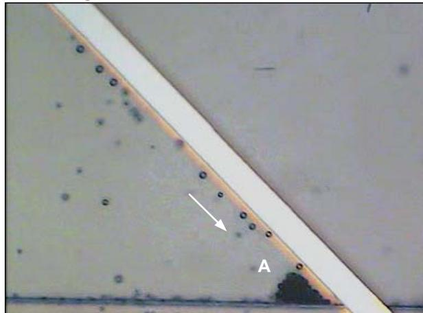
**Figure 5.** Particles were collected by the paired electrode array at the flowrate of  $50\mu\text{l/hour}$ .
