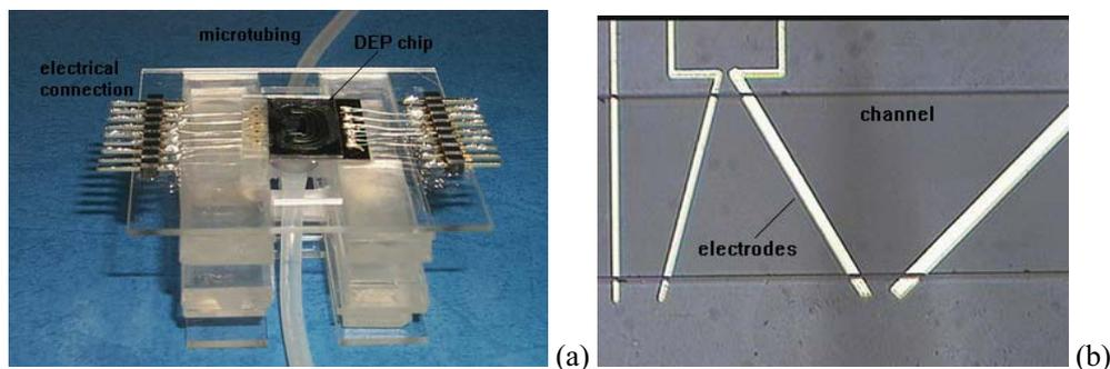
**Figure 3.** The microfabricated microfluidic system comprising 3-D deflector array. The insert (b) shows an array of electrodes of different width and aligning angles (top view).
