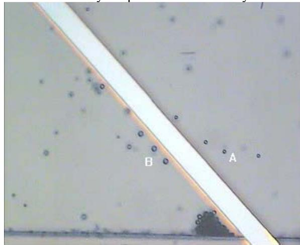
**Figure 6.** Particles of  $4.8\mu\text{m}$  penetrated the gate and were carried away by the flow.
