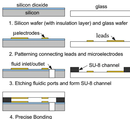
**Figure 2.** Microfabrication of the DEP device.
