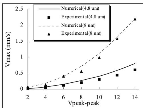
**Figure 4.** Threshold velocity for the latex particles with radius of 4.8 μm and 8.0 μm, respectively. The aligning angle was 45° and electrode width was 40 μm. Both the numerical values and measured values are shown.
