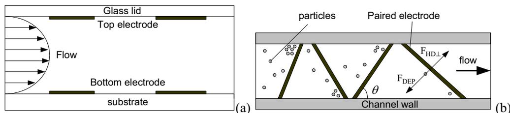
**Figure 1.** (a) Schematic diagram of paired microelectrode system (cross section). (b) The paired electrode system (top view) used for particle accumulation and separation in this paper.
