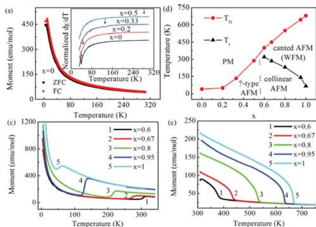
FIG. 2. (Color online) (a) ZFC and FC M-T curves of  $\text{DyMnO}_3$ . Inset: Temperature dependence of normalized  $d\gamma/dT$  for  $x \leq 0.5$ . (b) and (c) Temperature dependence of magnetic moment at low/high temperature range for  $0.5 < x \leq 1$ . (d) The Fe content dependence of the Néel temperatures ( $T_N$ ) and spin reorientation temperatures ( $T_r$ ). Speculated magnetic states are presented.
