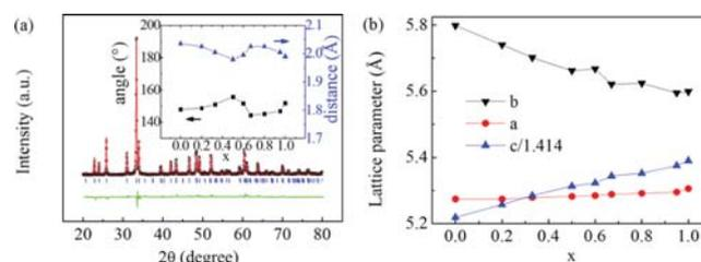
FIG. 1. (Color online) (a) XRD refinement calculation results on  $\text{DyMn}_{0.8}\text{Fe}_{0.2}\text{O}_3$  with  $R_p = 8.9\%$  (star symbols, experiment data; solid line, fitting data; short vertical solid lines, Bragg positions; fluctuation line at bottom, difference). Inset: Fe content dependence of Mn/Fe-O-Mn/Fe angles and Mn/Fe-O distances within  $ab$ -plane. (b) Lattice parameter dependence on Fe content.
