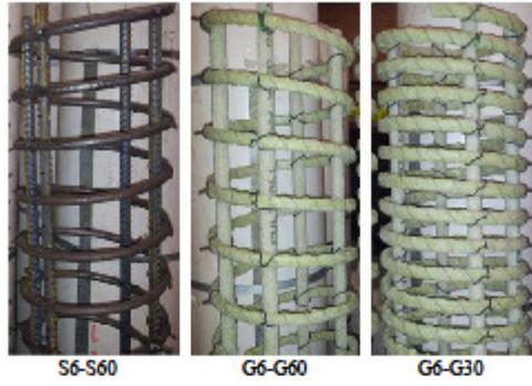
**Fig. 4. Reinforcement cages**
