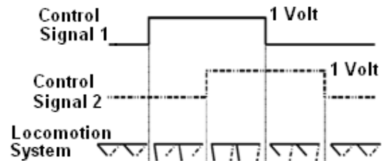
Figure 7: Actuation diagram of the actuators as the legs of the locomotion system.
