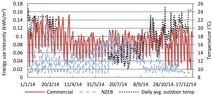
Fig. 8 HVAC energy use intensity comparison - 2014
