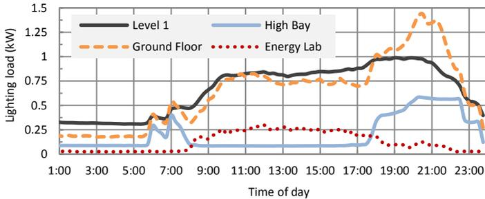
Fig. 5 SBRC lighting system average daily load profile
