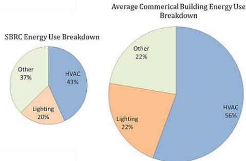
Fig. 9 Energy intensity of case study NZEB compared to typical commercial buildings.
