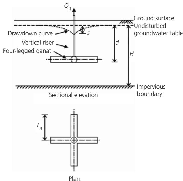
Figure 1. A typical four-legged qanat
