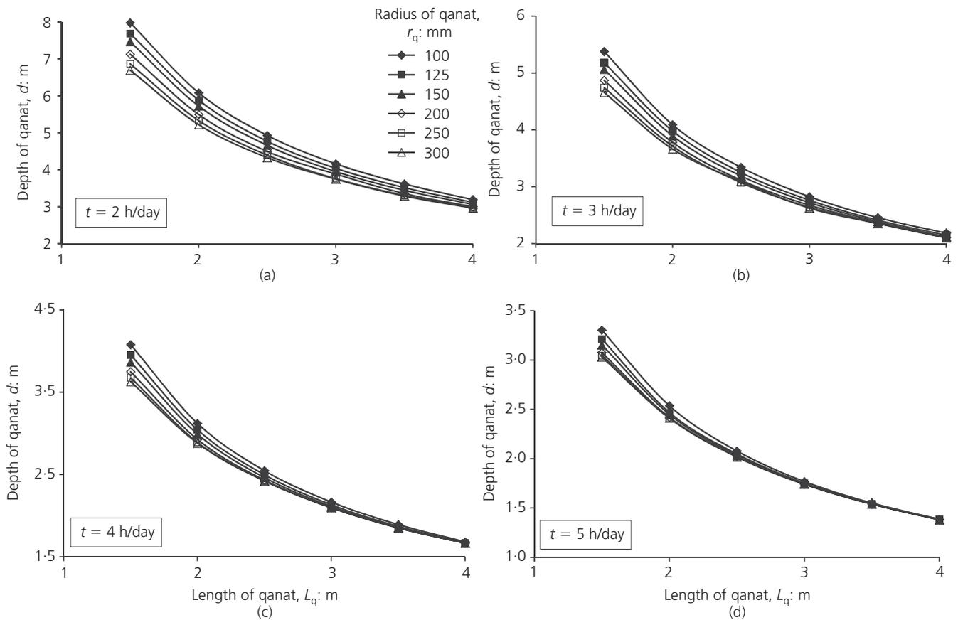
**Figure 6.** Variation of depth of qanat at base versus length of qanat leg for pumping duration (a)  $t = 2$  h/day, (b)  $t = 3$  h/day, (c)  $t = 4$  h/day and (d)  $t = 5$  h/day
