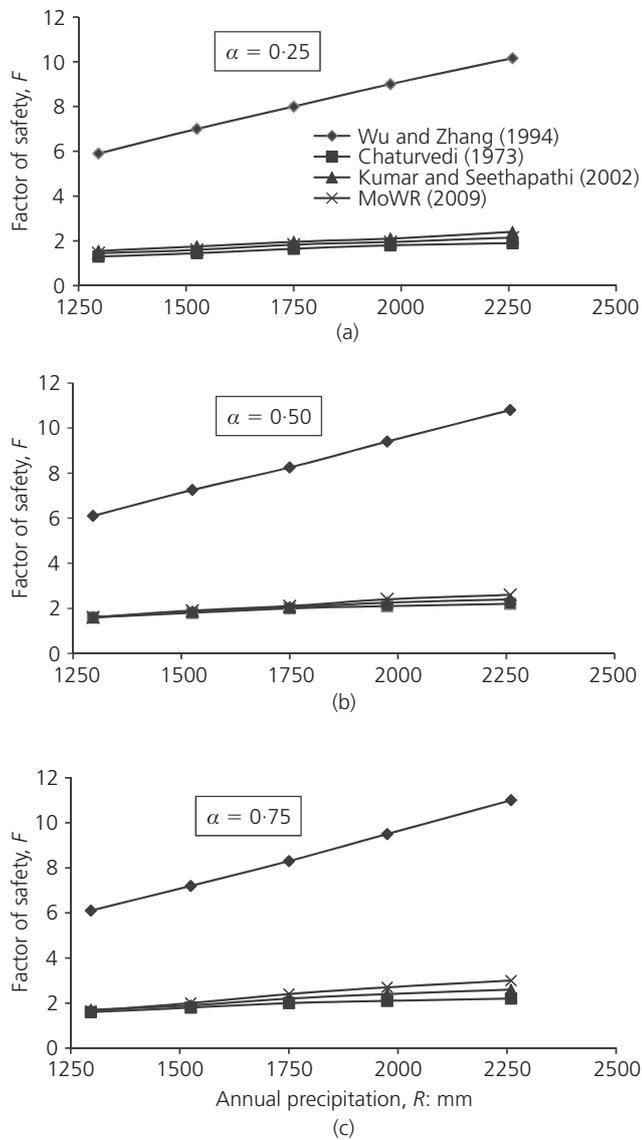
Figure 7. Variation of factor of safety  $F$  with annual precipitation  $R$  for (a)  $\alpha = 0.25$ , (b)  $\alpha = 0.50$  and (c)  $\alpha = 0.75$
