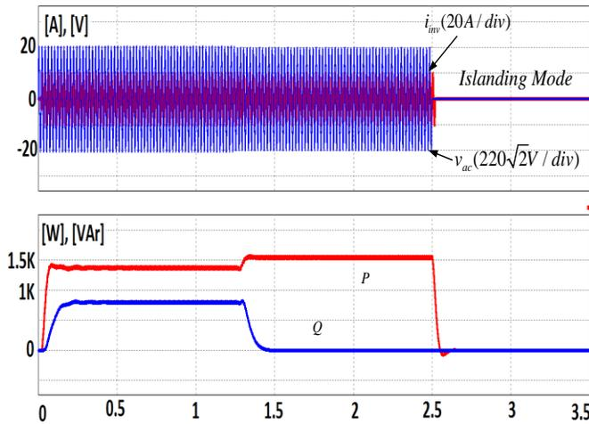
Fig. 12. Output current of the AC module during the Islanding Mode
