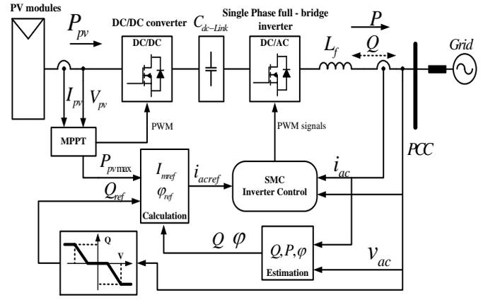
Fig. 2. Block diagram of the AC PV module.
