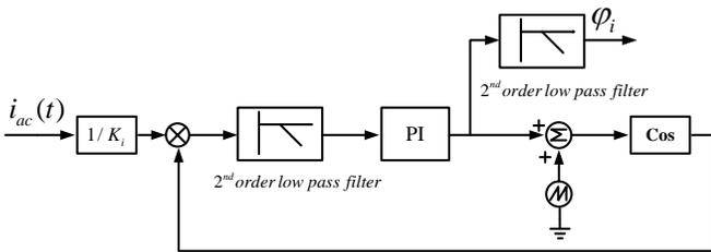
Fig. 5. Block diagram of the PLL blocks
