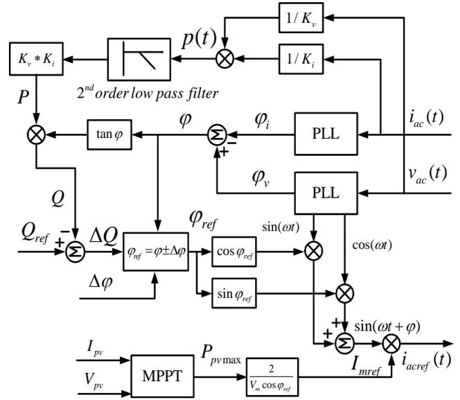
Fig. 3. Block diagram of the CRG.
