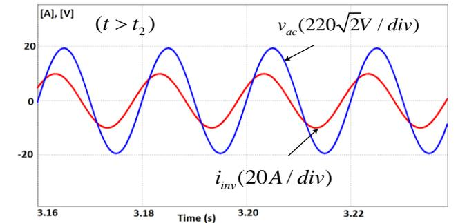
Fig. 10. The partially expanded waveforms of the current and grid voltage after time  $t_2$ .
