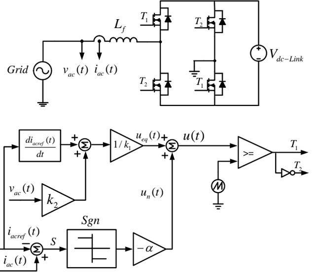
Fig. 6. Block diagram of the Sliding Mode Control (SMC) for controlling DC/AC inverter.
