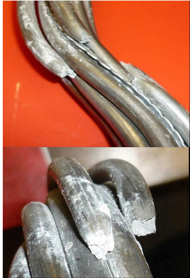
Figure 9. Cone and Cup strand failures.
