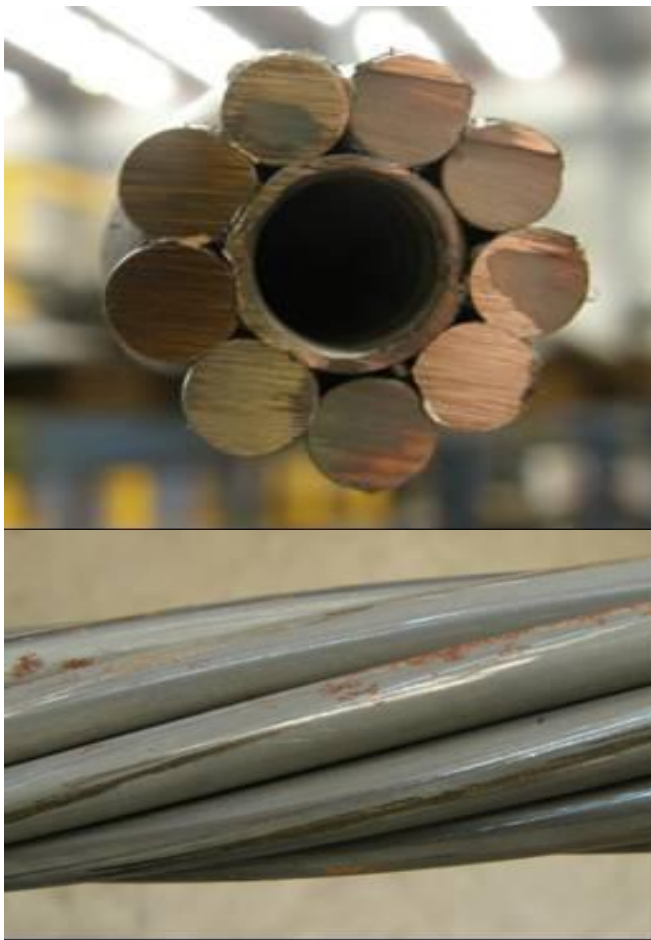
Figure 1. Cross section and side view of nine-strand TG cable bolt.
