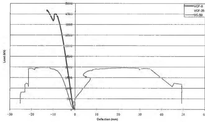
Fig. 11 Load-deflection for Specimens VCF-0, VCF-25 and VCF-50.
