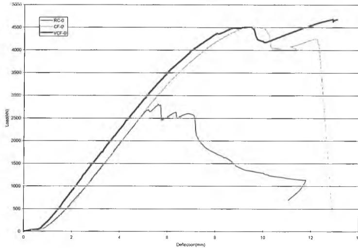
**Fig. 6** Load-deflection for Specimens RC-0, CF-0 and VCF-0.
