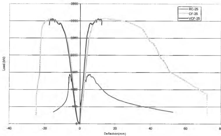
**Fig. 7** Load-deflection for Specimens RC-25, CF-25 and VCF-25.
