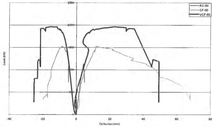
Fig. 8 Load-deflection for Specimens RC-50, CF-50 and VCF-50.
