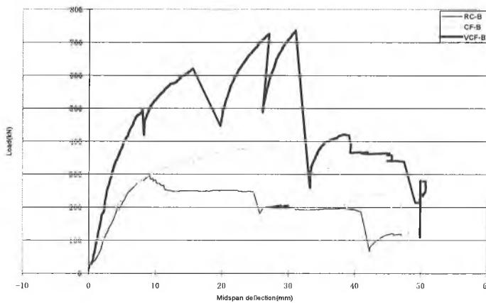
Fig. 12 Load-deflection for Specimens RC-B, CF-B and VCF-B.
