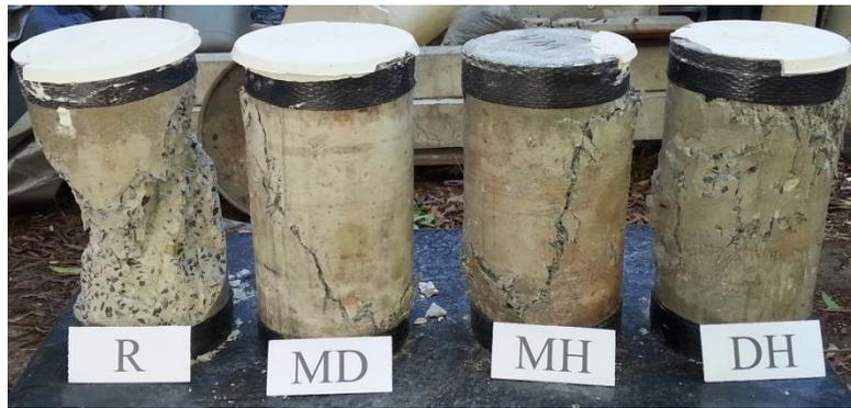
Figure 3. Typical failure modes.
