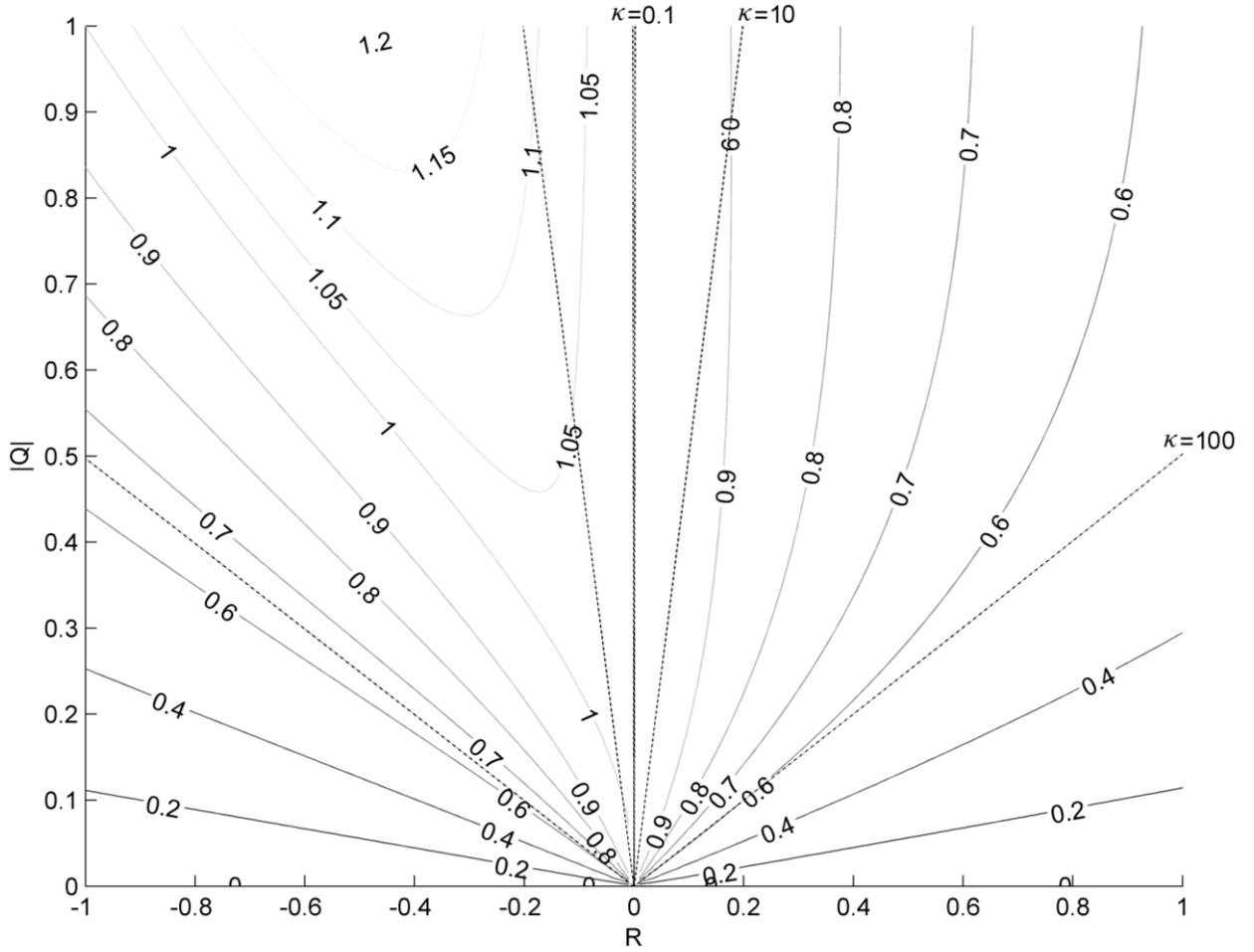
**Figure 2:** Maximum fixed OWC power capture ratio for compressible and incompressible flow; the dashed lines represents the frequency response for the case  $\kappa=0.1$ ,  $\kappa=10$  and  $\kappa=100$  as indicated;  $\zeta=0.01$ .
