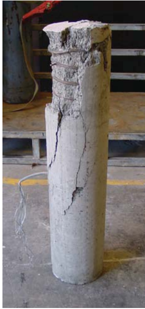
Figure 2 – Column N0 – Internal Reinforcement Only – e=0\text{mm}
