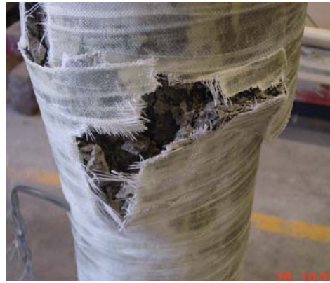
Figure 4 – Column G0 – Internal Reinforcement with Three Layers E-Glass – e=0\text{mm}
